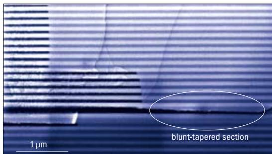
5–8 μm – that drive up the bias current required for a high modulation bandwidth. We avoid this pitfall by scaling down the VCSEL size. Although this leads to a power drop of 50%, it cuts power dissipation and increases the bandwidth, while maintaining acceptable optical losses.
