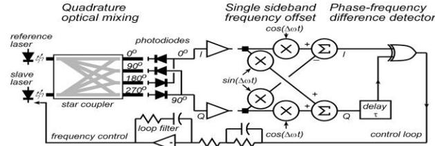
Fig. 1. The architecture of the OPLL consists of three parts: a photonic integrated circuit, an electrical integrated circuit and a loop filter.
