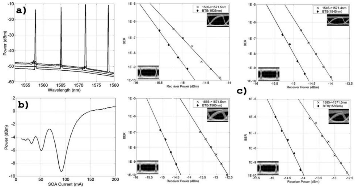
Figure 2 – a) Overlapped spectra of the device output wavelengths b) Typical electrical extinction curve for high SOA currents (SOA2 is biased at 200mA) c) BER results for conversion from 4 different input wavelengths
