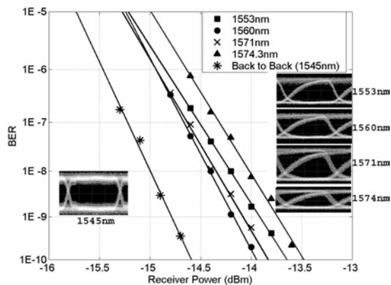
Figure 3 – BER results for conversion onto 4 device wavelengths
