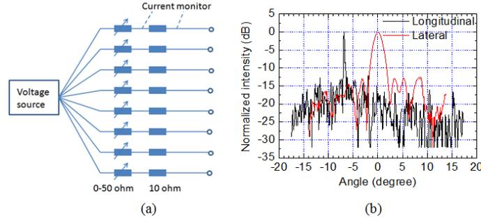
Fig. 2 (a) Schematic of the electrical setup for adjusting injection currents into the SOAs; (b) Optimized far-field pattern
