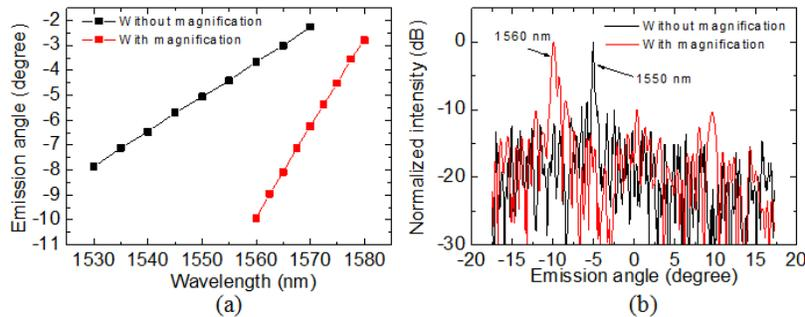
Fig. 3 (a) Peak position in the longitudinal direction versus wavelength; (b) Field distribution in the longitudinal direction.
