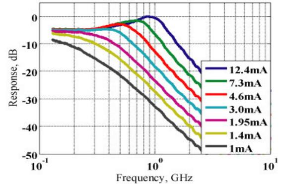
Figure 4. Link gain at different detected photocurrent values
