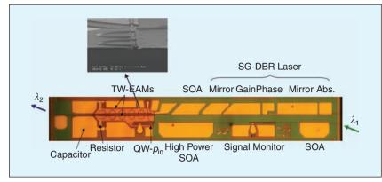
Figure 2. Transceiver/wavelength-converter: 2-stage-SOA-PIN Receiver and SGDBR-TW/EAM Transmitter.
