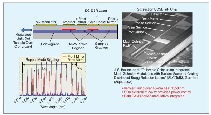
Figure 1. Widely-Tunable SGDBR-SOA-Modulator PIC.
