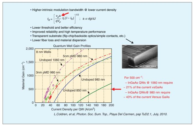
Figure 5. The case for 980-1100 nm (strain/GaAs).
