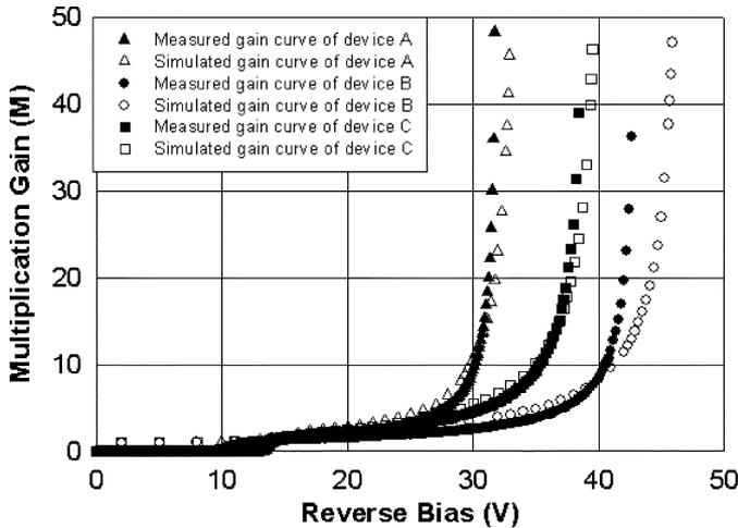
Fig. 4. Measured and simulated gain as a function of reverse bias voltage for devices A, B, and C.
