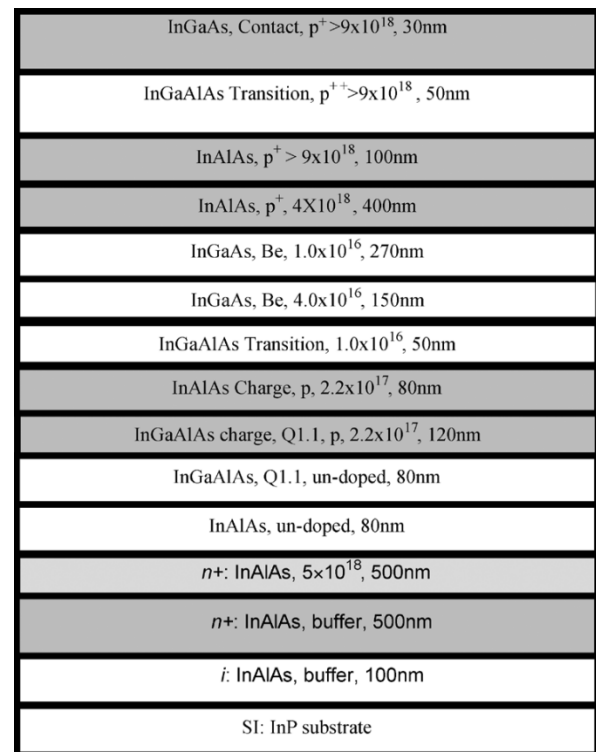
Fig. 1. Schematic layer structure of the SACM APD.
