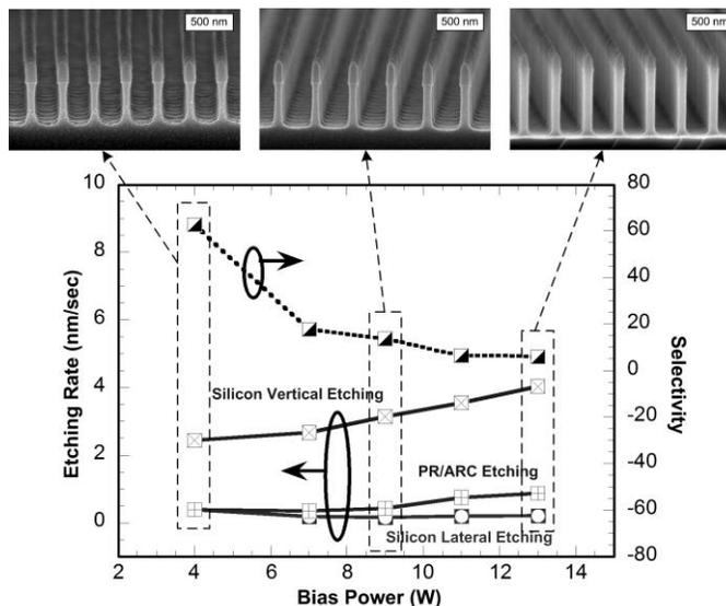
Figure 4 Etching rate of SDRIE and the sidewall angle of resultant patterns under different flow composition of SF<sub>6</sub> and C<sub>4</sub>F<sub>8</sub> gas mixture
