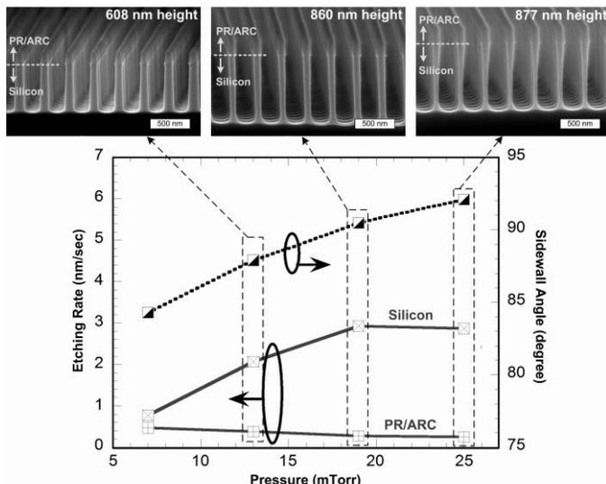
Figure 3 Silicon etching rate and SNWA sidewall angle against the chamber pressure
