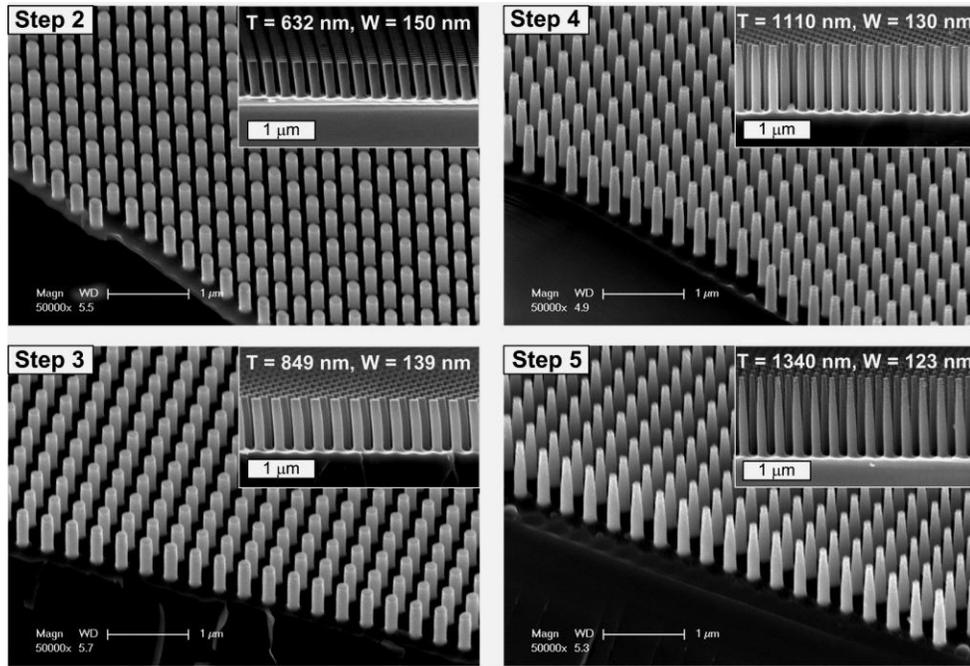
Figure 5 SEM views of resultant profiles after each step of the modified SDRIE with linearly-changed  $C_4F_8/SF_6$  gas flow
