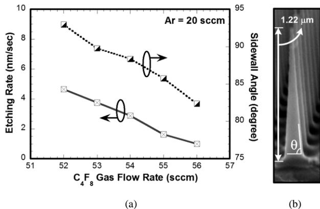
Figure 2 Etching rate and sidewall angle, as defined in (b), for different C<sub>4</sub>F<sub>8</sub> gas flow rate.
