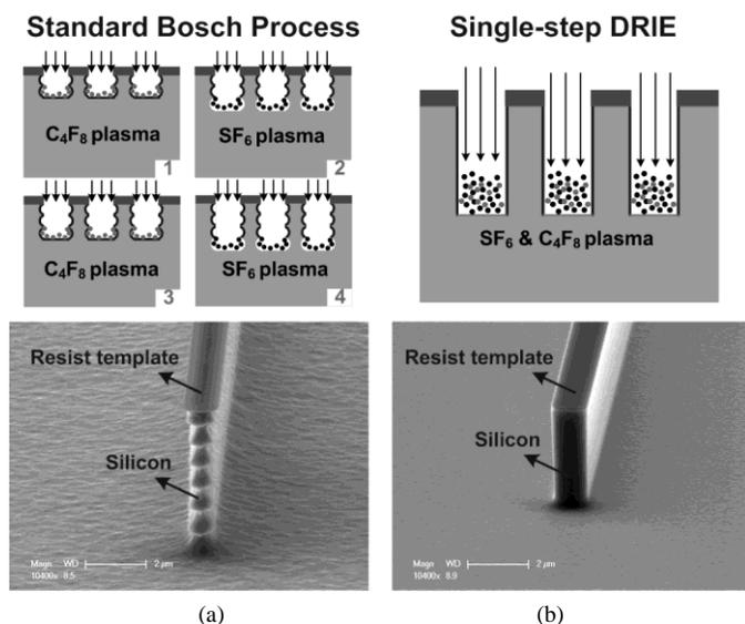
Figure 1 Schematic of etching process and the resultant profiles for (a) Bosch and (b) SDRIE process
