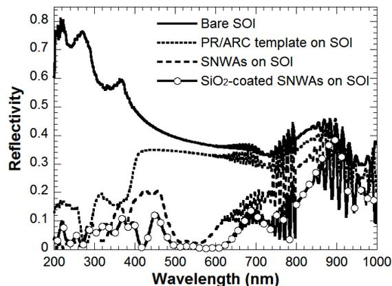
Figure 10 Measured reflection spectra of bare SOI, 250 nm tall PR/ARC templates on SOI, 700 nm tall square SNWAs on SOI, and the 700-nm tall SNWAs coated with a 186 nm thick  $SiO_2$  film
