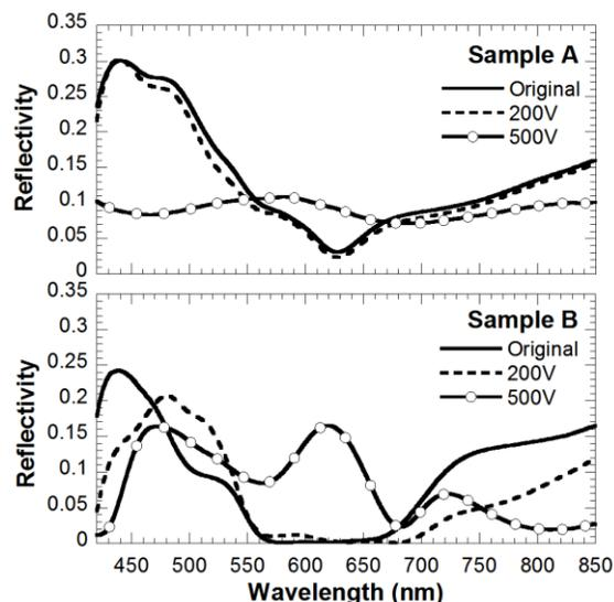
Figure 9 Measured reflection spectra of Sample A and B in Figure 7 after post argon plasma treatment with different RF bias voltage.
