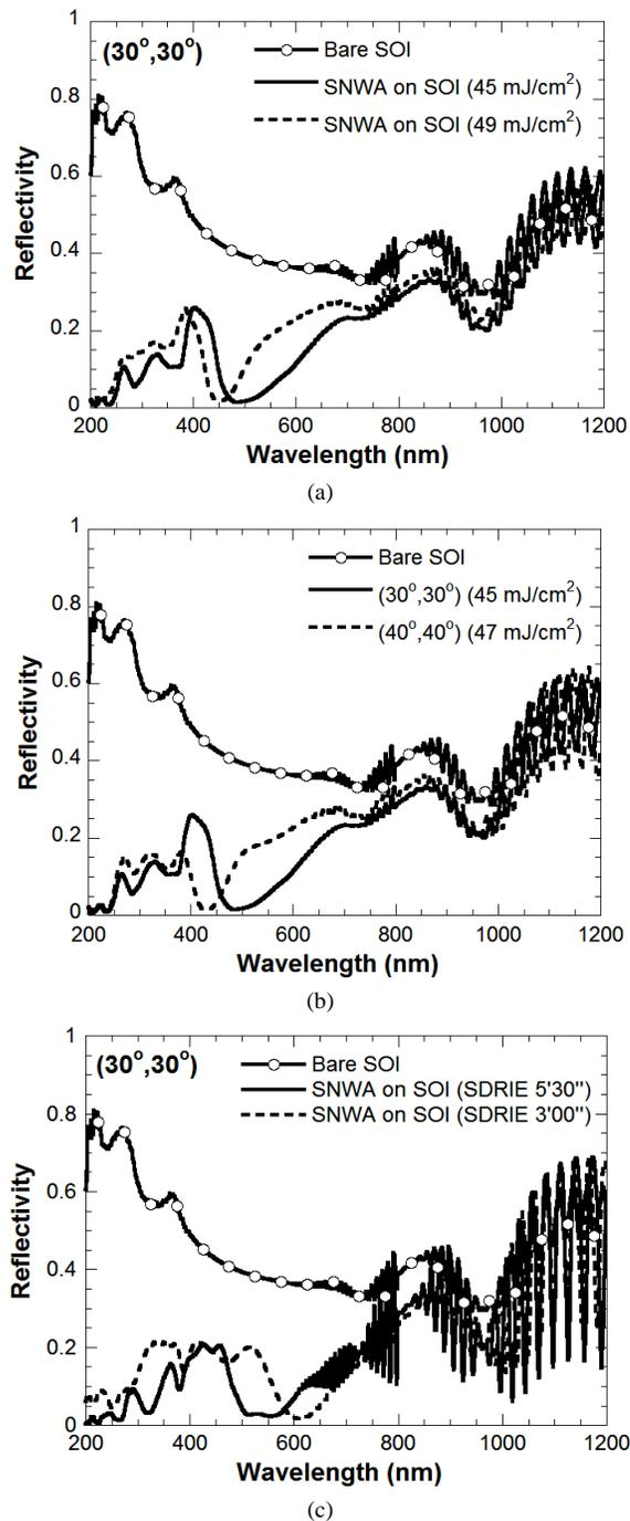
Figure 11 (a) Measured reflection spectra of 330 nm spaced square SNWAs on SOI substrate with different exposure time during holography for obtaining different pillar widths. (b) Measured reflection spectra of SNWAs on SOI substrate with different lattice constants. (c) Measured reflection spectra of square SNWAs on SOI substrate with different SDRIE etching time for obtaining different pillar heights.
