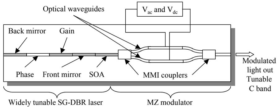
Fig. 13: Schematic overview of integrated SGDBR-SOA-MZM device.
