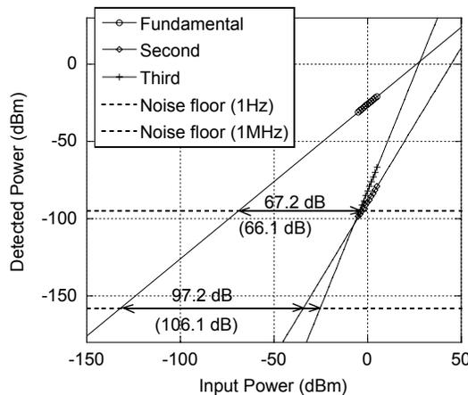
Fig. 7: Measured power of noise floor, fundamental, second and third order intermodulation products at 1552 nm, for  $-5\text{ dBm}$  to  $5\text{ dBm}$  input RF power,  $6.3\text{mW}$  optical power and  $-1.1\text{V}$  EAM bias. Broadband spurious-free dynamic range is also shown in 1Hz and 1MHz bandwidth.
