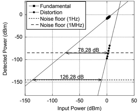
Fig. 8: Measured power of noise floor, fundamental and third order intermodulation products at 1552 nm, for  $0\text{ dBm}$  to  $5\text{ dBm}$  input RF power,  $0.96\text{mW}$  optical power and  $-2.5\text{V}$  EAM bias. Sub-octave spurious-free dynamic range is also shown in 1Hz and 1MHz bandwidth.
