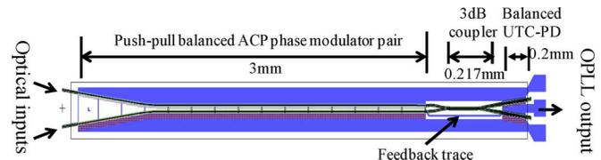
Fig. 1. ACP-OPLL photonic integrated circuit.
