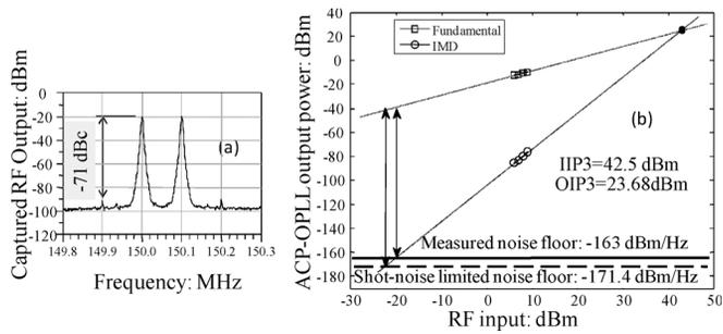
Fig. 5. Distortion measurements at 150 MHz. (a). Captured RF spectrum with 7 dBm RF input. (b) The third order intercept point measurement. The ACP-OPLL output is 7.78 dB higher than the spectrum analyzer reading.
