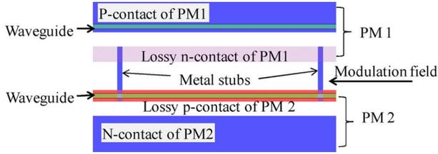
Fig. 2. A section of push-pull ACP phase modulator.
