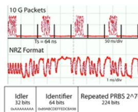
Fig. 2. Transmitted packet stream, NRZ format, and packet format.
