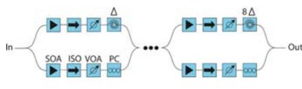
Fig. 4. Feed forward 4-stage optical packet synchronizer.
