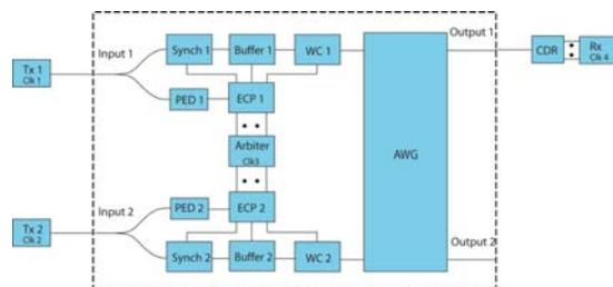
Fig. 1. Asynchronous 2x2 optical packet switch architecture.
