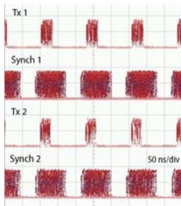
Fig. 7. Screenshots of transmitted and synchronized packets.
