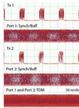
Fig. 8. Screenshots of transmitted, synchronized/buffered, and TDM packets.
