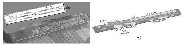
Figure 1 – (a) 40 Gbps MZI-SOA packet forwarding chip (PFC) electron micrograph (b) PFC schematic (c) 40 Gbps separate absorption and modulation (SAM) tunable wavelength converter
