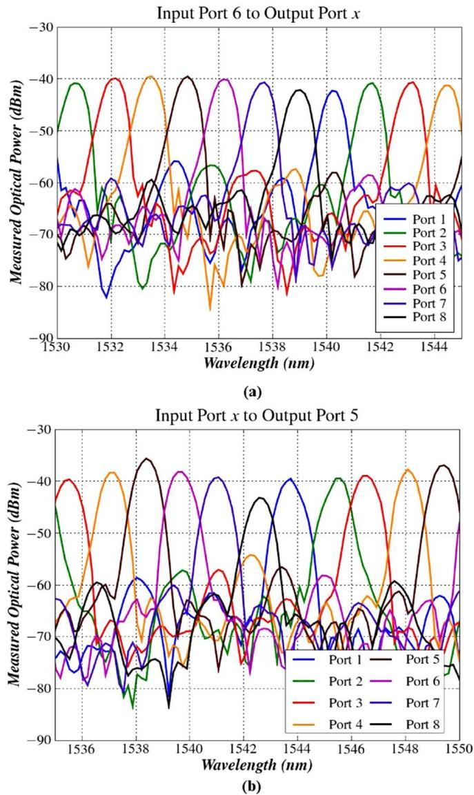
Fig. 8. Output ASE response of the integrated AWGR: (a) measured optical output from all output ports using input wavelength converter #3; (b) measured optical output from output port #2 using each input wavelength converter.
