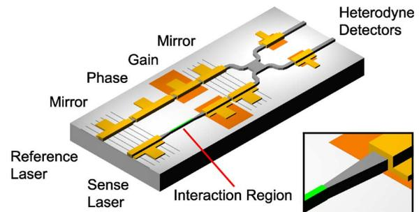
Fig. 1. Schematic of the intracavity sensor composed of two SG-DBR lasers and a heterodyne spectrometer utilizing a  $2 \times 2$  combiner and quantum-well photodetectors. The interaction region of the sensing laser, shown in the inset, has no dielectric layer on the ridge and is narrowed to increase the modal overlap with the cladding index.
