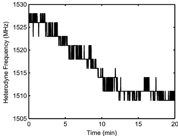
Fig. 5. Heterodyne frequency stability of 0- $\mu\text{m}$  device. Device is held at a constant bias of 91 and 80 mA on the reference and sensing laser gain sections, respectively, and 3 mA on the reference laser phase section. Standard deviation of signal is 5.9, 1.5, and 0.4 MHz for 20-, 10-, and 1-min intervals, respectively.
