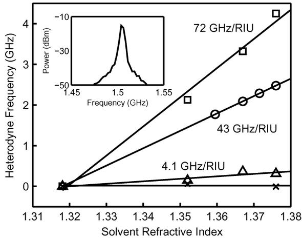
Fig. 4. Comparison of heterodyne shift for devices with different ridge widths: 0  $\mu\text{m}$  ( $\square$ ), 1  $\mu\text{m}$  ( $\circ$ ), 3  $\mu\text{m}$  ( $\triangle$ ), and reference ( $\times$ ). Temperature effects, corresponding to 7% of the raw values for the 0- $\mu\text{m}$  device, have been removed from the data. Inset shows a typical heterodyne signal for 0- $\mu\text{m}$  device with a 3-dB linewidth of 3.6 MHz.
