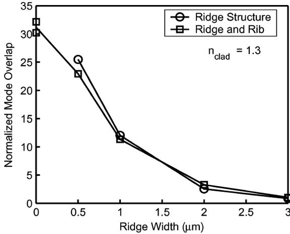
Fig. 2. Normalized modal overlap for narrowed ridge structures. The overlap values are normalized to the value for a 3- $\mu\text{m}$ -wide ridge ( $\Gamma_{xy} = 0.012\%$ ). The device with the highest overlap, the 0- $\mu\text{m}$  ridge width structure, has the p-InP upper cladding completely removed in the sensing region.
