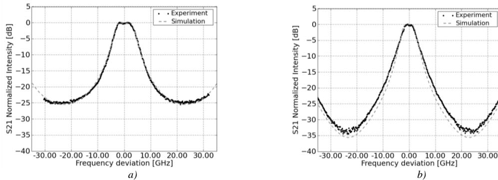
Fig.3 Experimentally measured filter responses from cascaded filter stages, simulations using Eq.(1) and (2) are superimposed. a) 2<sup>nd</sup> order flat-top band-pass filter response and b) 3<sup>rd</sup> order filter - 2<sup>nd</sup> order flattop band-pass filter with a zero placed half way in between the pass-bands. Data was normalized in frequency and intensity.
