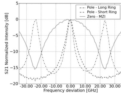
Fig.2 a) Optical image of wire bonded device with 4 cascaded filter stages. b) Experimental filter responses from a single stage filter, normalized in frequency and intensity.
