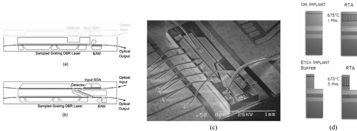
**FIGURE 1.** (a) Top view schematic of the device with discrete detector/modulator architecture, where the transmitter device used in this work is shown with dark outline. (b) Top view schematic of the interconnected device used in the wavelength converter work. (c) Electron micrograph of the completed wavelength converter device mounted on carrier (d) Illustration of the intermixing processing platform used in this work.
