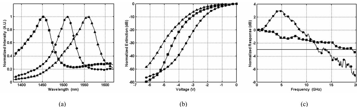
**FIGURE 2.** (a) Photoluminescence spectra of active section (triangles), modulator section (circles), and passive sections (squares). (b) DC extinction of a 175  $\mu\text{m}$  modulator for wavelengths of 1558 nm (circles), 1570 nm (squares), and 1580 nm (triangles). (c) Electrical to optical frequency response of the transmitter device (squares) and optical to optical frequency response for wavelength converter device.
