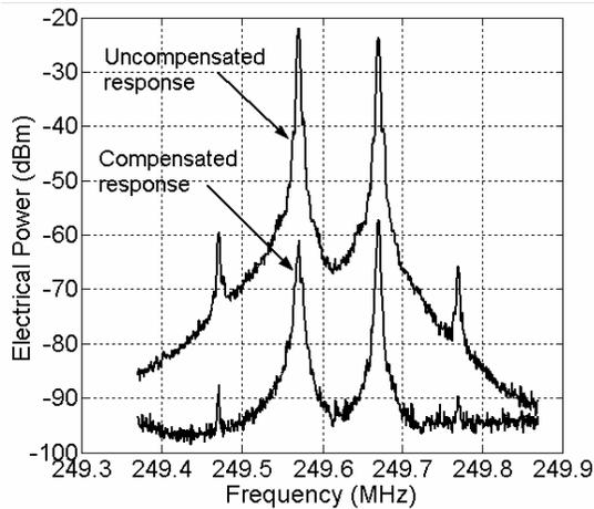
Fig 2. Compensated and uncompensated balanced detector response. Electrical drive power is -15 dBm and -10 dBm to the InGaAsP and LiNbO<sub>3</sub> modulators respectively
