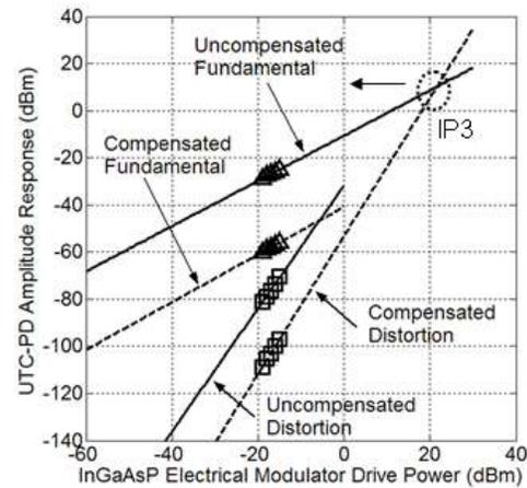
Fig 3. Fundamental and third order distortion in the amplitude response of the UTC-PDs for both compensated and uncompensated experiments.
