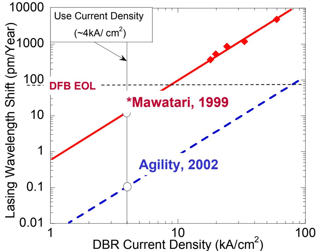
\*Mawatari et al, "Lasing Wavelength Changes Due to Degradation in Buried Heterostructure DBR Laser", Journal of Lightwave Technology, v.17, no.5 1999
