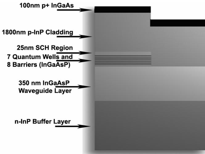
Fig. 2. Offset quantum well epitaxial structure - active-passive interface
