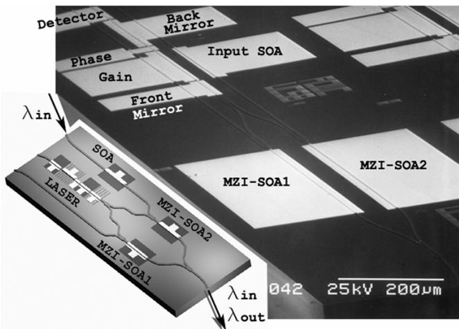
Fig. 1. SEM image and a schematic of the device
