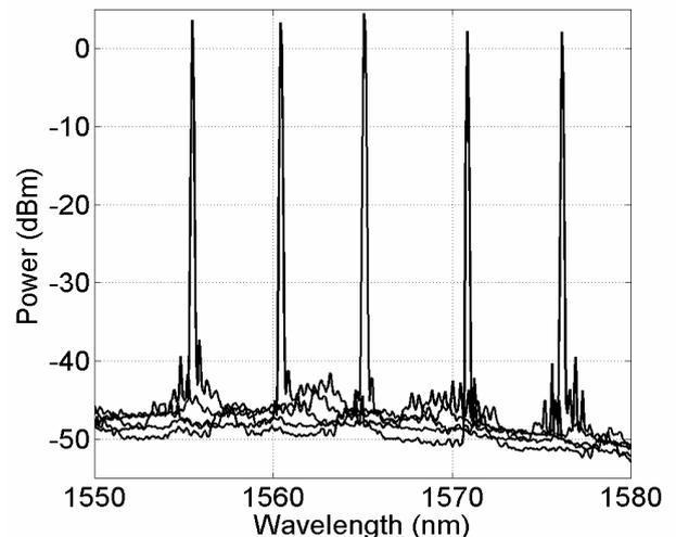
Figure 2 – Example overlapped spectra of the AOWC
