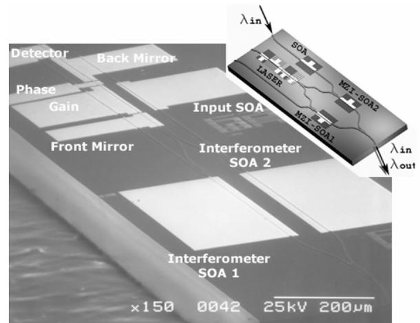
Figure 1 - SEM image of the wavelength converter
