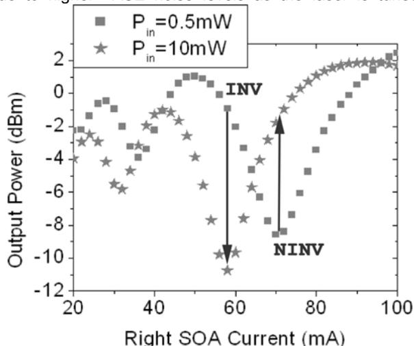
Figure 6 - Electrical transfer functions vs input signal power
