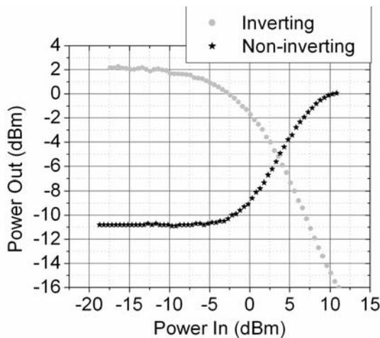
Figure 3 – Typical optical static transfer functions
