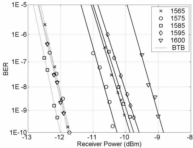
Figure 5 - BER curves for 5 input wavelengths
