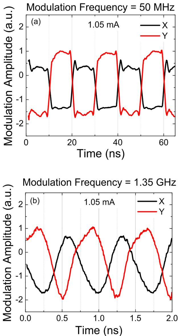
FIG. 4. Time domain modulation response for VCSEL in X and Y polarizations for modulation frequency of (a) 50 MHz, (b) 1.35 GHz at 1.05 mA bias current.
