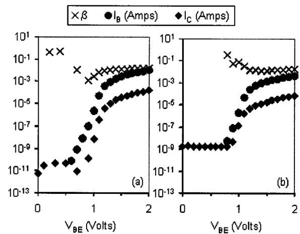
FIG. 3. Room-temperature Gummel plots for the  $n$ -AlGaAs- $p$ -GaAs- $n$ -GaIn HBT fused (a) at 600 °C and (b) at 750 °C.
