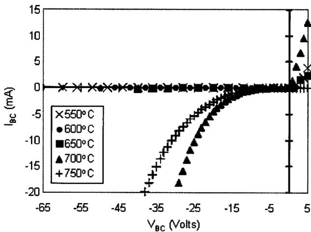
FIG. 1. Room-temperature  $I-V$  characteristics for the  $p$ -GaAs- $n$ -GaN base-collector diode, fabricated via wafer fusion at systematically varied temperatures (550–750 °C for 1 h).
