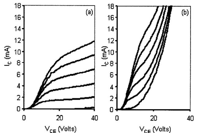
FIG. 4. Room-temperature common-emitter characteristics for the  $n$ -AlGaAs- $p$ -GaAs- $n$ -GaIn HBT fused (a) at 600 °C and (b) at 750 °C.  $I_B$  step size = 2 mA.
