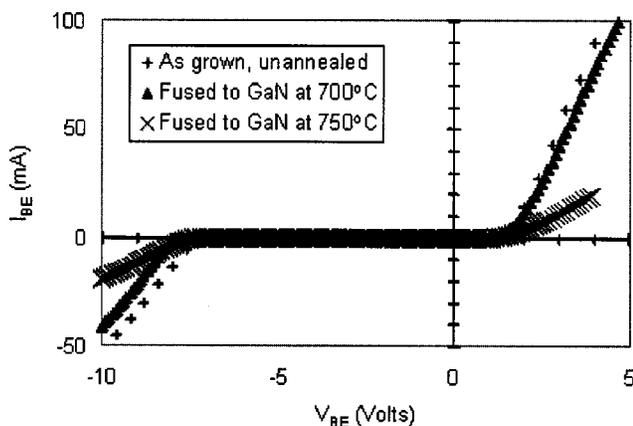
FIG. 2. Room-temperature  $I-V$  characteristics for the  $p$ -GaAs- $n$ -AlGaAs base-emitter diode as grown, and after this structure is wafer-fused to an  $n$ -GaIn collector at 700 and 750 °C.
