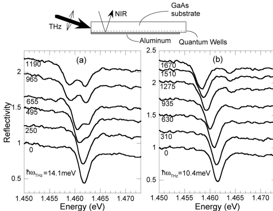
Fig. 1. Reflectivity spectra at 10 K for a series of THz powers at (a)  $\hbar\omega_{\text{THz}} = 14.1$  meV and (b)  $\hbar\omega_{\text{THz}} = 10.4$  meV. The spectra are offset and labelled according to the THz power (in Watts). A schematic of the sample and experimental geometry is displayed above.
