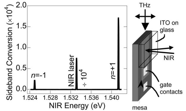
FIG. 2. Sideband spectrum taken at  $\sim 11$  K with  $\omega_{THz} = 2.0$  THz (8.2 meV) at  $\sim 730$  kW/cm<sup>2</sup>. The NIR laser signal is divided by  $\sim 1 \times 10^4$ .  $E_{bias} = 5.8$  kV/cm. The experimental geometry is to the right of the figure.
