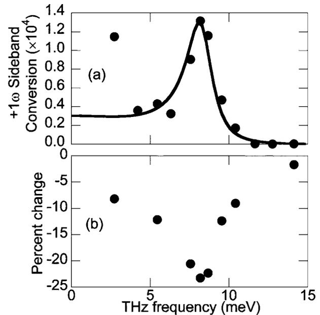
FIG. 5. (a) Peak values of the  $n=+1$  sideband resonance spectra (solid dots) for the doped sample and the peak values of the  $\chi^{(2)}$  model curves (solid line) plotted vs  $\omega_{THz}$ . (b) Percent change in the integrated PL of the doped sample with the THz field on at an intensity of  $\sim 40 \text{ kW/cm}^2$ .
