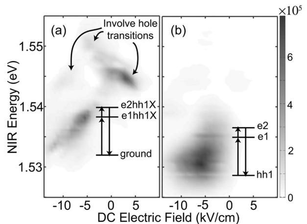
FIG. 3. The  $n = +1$  sideband resonance maps of (a) the undoped and (b) doped samples at  $\omega_{THz} = 2.0$  THz (8.2 meV), taken by varying  $\omega_{NIR}$  and  $E_{bias}$ , while always measuring the  $n = +1$  sideband. The sideband conversion for each point is represented on a grey scale, displayed on the right. The maps were taken at  $\sim 12$  K with a THz intensity of  $\sim 18$  kW/cm<sup>2</sup> and a NIR intensity of  $\sim 25$  W/cm<sup>2</sup>.
