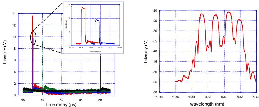
Fig. 2. **Left:** Different time delay values correspond to four discrete FBGs. The delay time differences between the FBG1 and others are 29ns, 1.06 $\mu$ s, and 7.02 $\mu$ s, respectively. The inset is the detail of the first two reflected pulse. **Right:** The reflection spectrum from the four FBGs. The non-uniform peak intensity of each FBG is here mainly due to interconnect loss.
