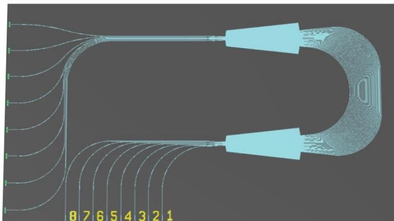
**Need short mode transition elements to maximize coupling between waveguide regions**
