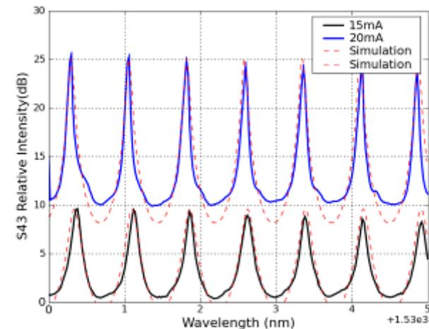
Measured and Simulated Resonator Pole Response – Varied Ring SOA Current (curves shifted for clarity)
