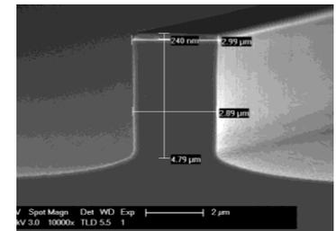
Deeply Etched Waveguide
