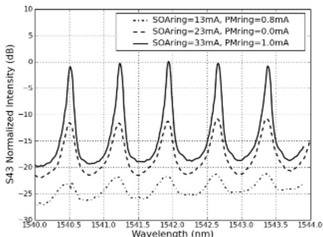
S43 Pole response tuned in amplitude
