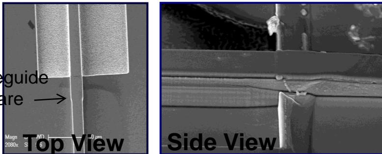
Surface Ridge to Deeply Etched Waveguide Transition
