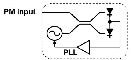
Costa's Loop for BPSK, QPSK demodulation
