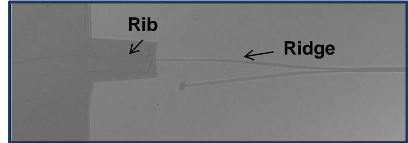
Surface Ridge to Buried Rib Butt Couple Transition
