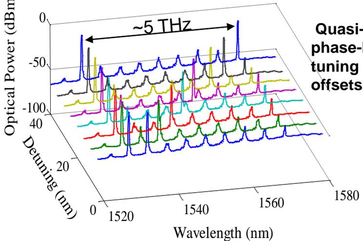
Quasi-continuous phase-locked digital tuning up to 5 THz offsets possible
