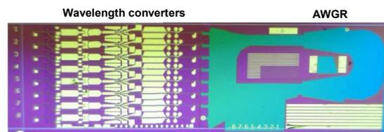
Fig. 3. 8 x 8 all-photonic space switch employing wavelength converters and a passive dispersive AWGR filter.
