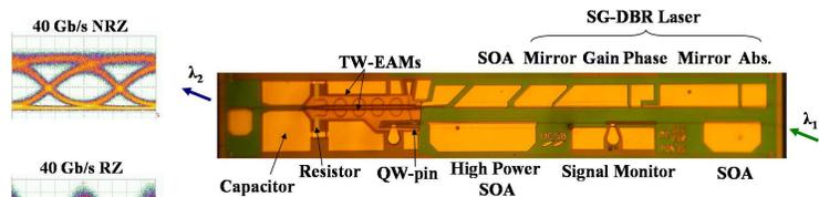
Fig. 2. Photocurrent-driven wavelength converter and outputs for both NRZ and RZ input data @ 40 Gb/s.
