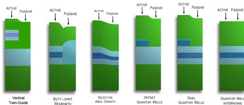
Fig. 1. Schematic waveguide cross sections of six active-passive integration platforms. All have been used in commercial products.
