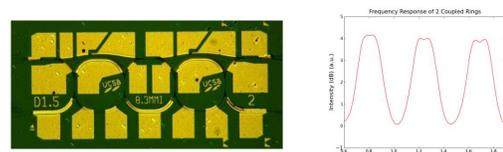
Fig. 4. Programmable lattice filter and 2-pole IIR response.
