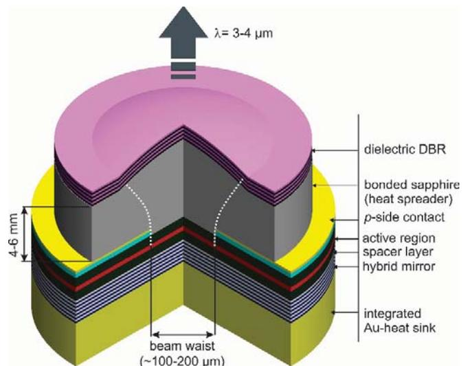
Fig. 1 Sketch of an electrically-pumped VECSEL with an episcide down configuration for the 3-4  $\mu\text{m}$  wavelength range. Several device components are indicated.
