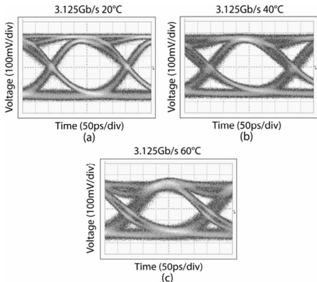
Fig. 5 Eye diagrams for 3.125Gb/s operation at 20°C (a), 40°C (b), and 60°C (c). Extinction is >8dB up to 60°C with a drive voltage of only 800mV.
