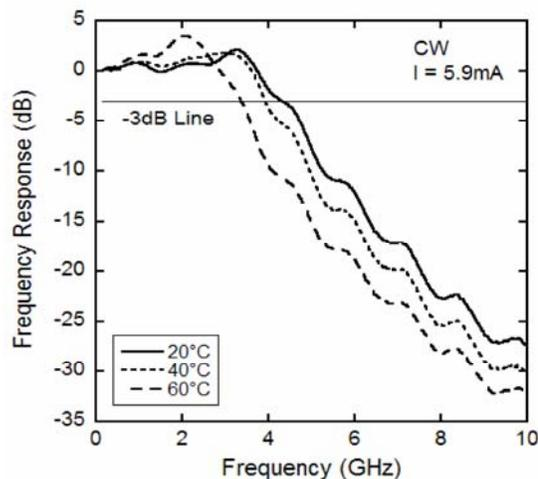
Fig. 4. Small-signal frequency response for VCSEL with  $8\mu\text{m}$  aperture diameter at  $20^\circ\text{C}$ ,  $40^\circ\text{C}$ , and  $60^\circ\text{C}$  at  $5.9\text{mA}$ ,  $5.2\text{mA}$ , and  $4.9\text{mA}$  drive currents, respectively.
