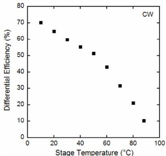
Fig. 3. CW Differential Efficiency vs. Stage Temperature showing differential efficiency of 64% at RT and over 50% at  $50^\circ\text{C}$ .
