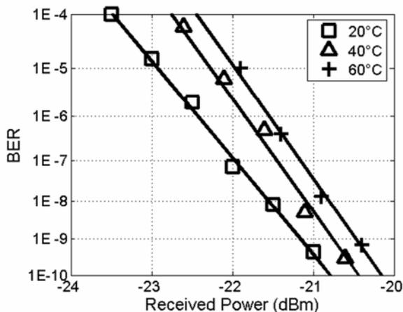
Fig. 6. BER vs. Received Power for 3.125Gb/s modulation at 20°C, 40°C, and 60°C for a  $2^{31}-1$  PRBS demonstrating error-free operation. Extinction ratio is >8dB up to 60°C. Measurements were performed back-to-back.
