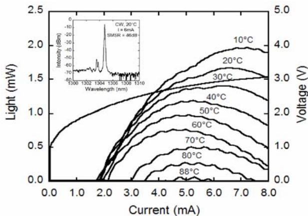
Fig. 2. CW LIV curves for bottom-emitting  $1.3\mu\text{m}$  VCSEL with  $8\mu\text{m}$  aperture for various stage temperatures. Inset lasing spectrum shows emission at  $1.305\mu\text{m}$  and  $46\text{dB}$  SMSR. Ripples on LI curve are due to substrate reflections from bottom-emitting device.
