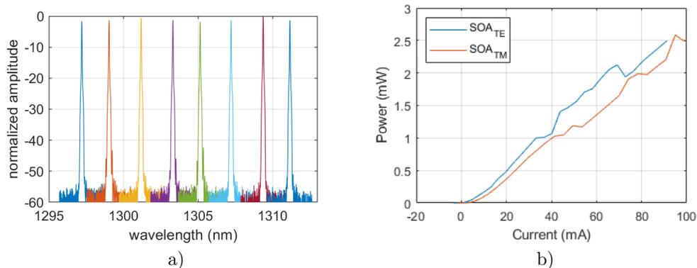
Figure 2: a) Normalized laser frequency spectrum on the OSA showing wavelength tunability across 2 nm spaced wavelength channels. b) Polarization channel SOA injection current versus output facet power. The SOA not being swept was biased at absorption in both LI measurements.
