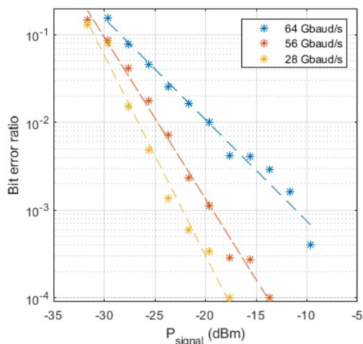
Figure 4: Sensitivity curves at 64, 56, and 28 Gbaud for received signal power per photodetector versus BER.
