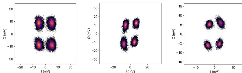
Figure 5: QPSK constellations at 64, 56, and 28 Gbaud for lowest BER of each baudrate.
