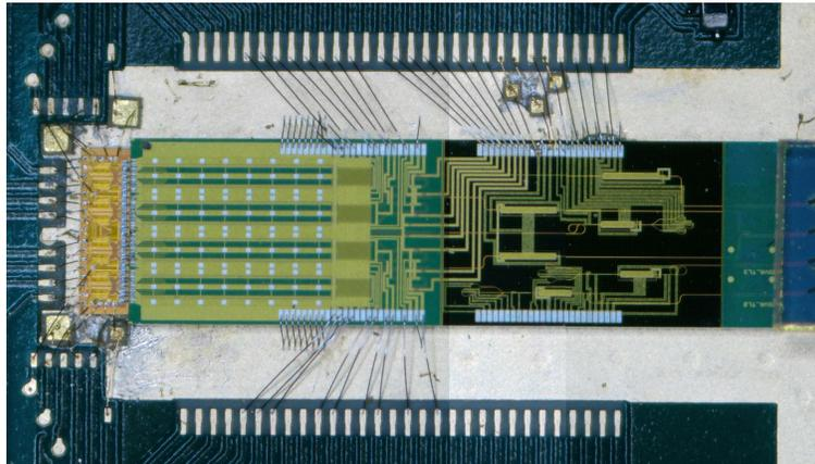
Figure 1: Micrograph of the 1.3 mm long driver on the left and 12.5 mm long PIC on the right. Both chips are 3 mm wide and had several DC traces bonded to small decoupling capacitors.
