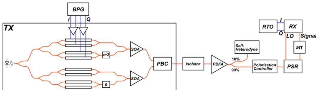
Figure 3: Block diagram of the transmitter with on-chip laser and self-homodyne test setup. Polarization carrier multiplexing was achieved by biasing the LO branch to the peak and the QPSK signal to null output power.
