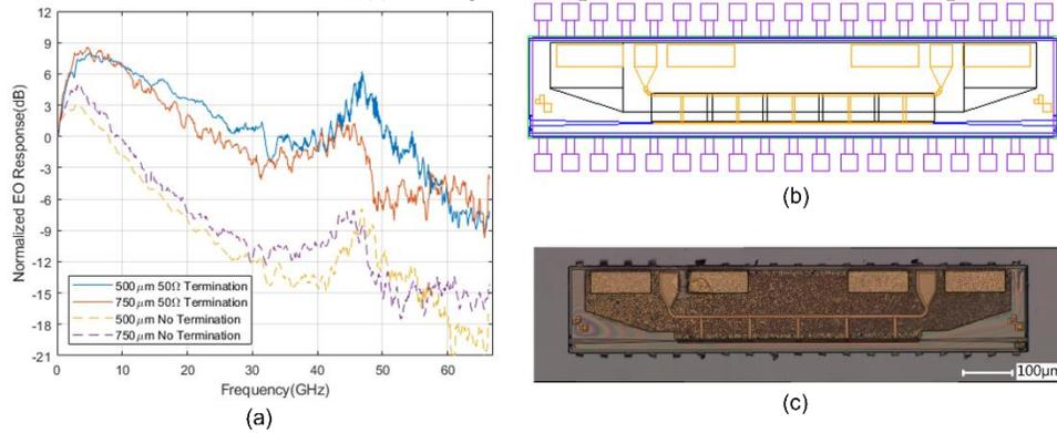
Fig. 3. (a) Bandwidth measurements of discrete TW modulators; (b) CAD layout of MTP TW EAM (c) TW modulator printed onto bare Si.
