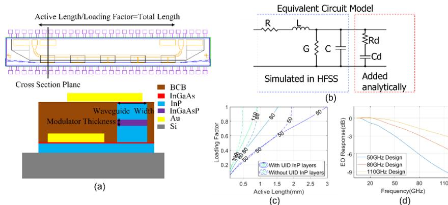
Fig. 1. (a) Cross section of designed microstrip modulator transferred to silicon; (b) Distributed circuit model for loaded microstrip transmission line; (c) Design space for modified and conventional epitaxy for several bandwidth targets; (d) Simulated response for 2.6 mm, 1.2 mm and 0.6 mm traveling wave modulators with a 20  $\Omega$  load impedance and 100% loading.
