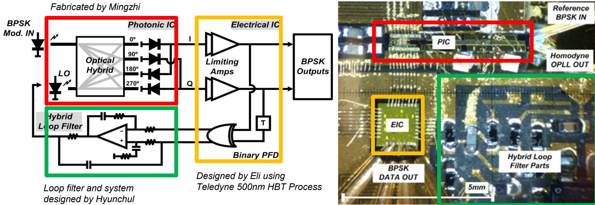
**Photonic IC:** SGDBR laser, optical hybrid, and un-balanced PDs
