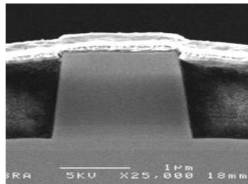
Deep etched waveguide
