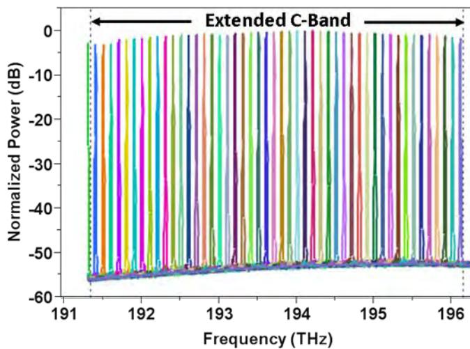
Typical laser output spectrum
