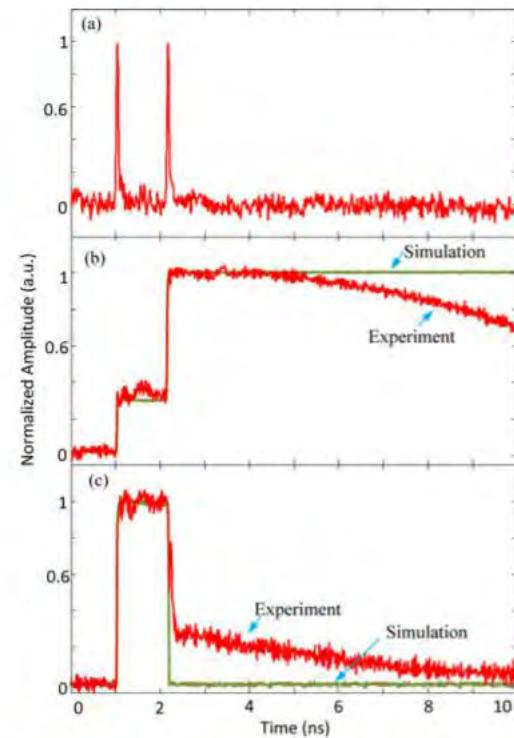
Fig. 8. The experimental results. (a) The input in-phase doublet pulse, (b) the integral of the in-phase doublet pulse, and (c) the integral of the out-of-phase doublet pulse.
