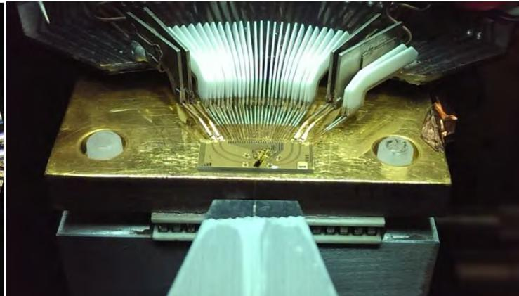
Wafer-Level Electrical and Optical Measurements
