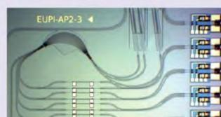
tunable laser with integrated MZI modulator
