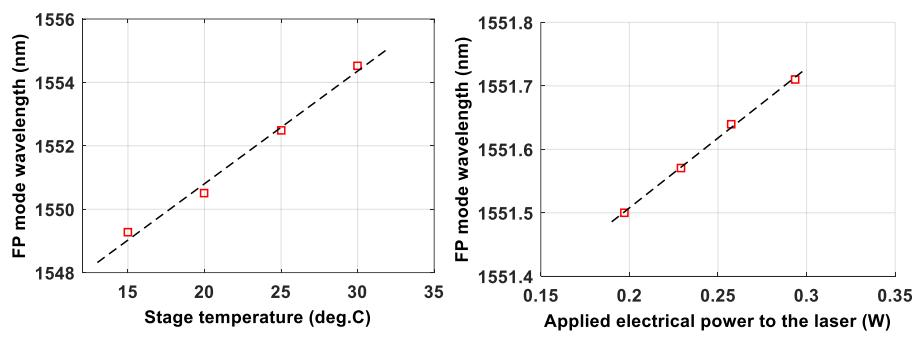
Thermal impedance =  $18.63 \text{ } ^\circ\text{C/W}$
