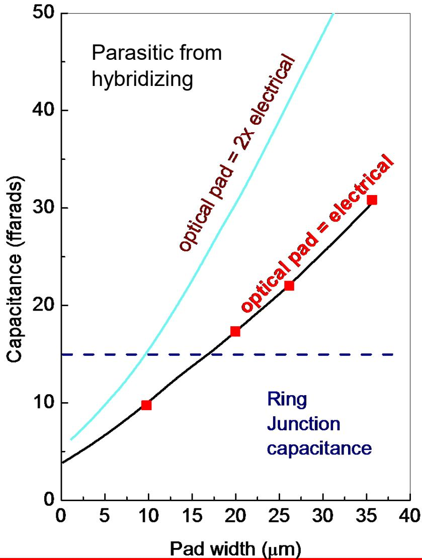
**Hybrid approach** parasitics become smaller than device junction as pad shrinks
