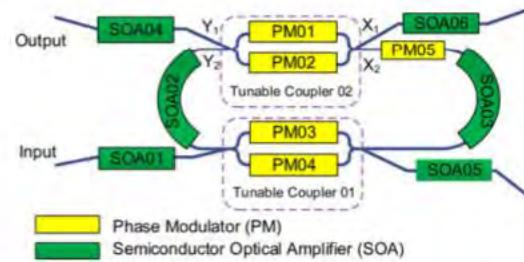
Fig. 2. The schematic of the proposed on-chip photonic temporal integrator based on a microring resonator.
