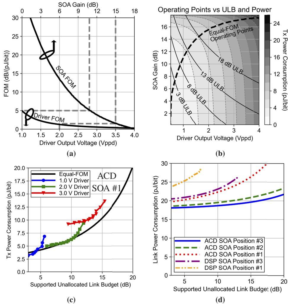
**Fig. 5.** Driver and SOA FOMs vs output voltage and gain operating points (a). Optimal equal-FOM operating points plotted with Tx power consumption and ULB contours for an ACD-based link with SOA in position #2 (b). Equal-FOM curve for an ACD-based link with SOA in position #1 vs. time-domain simulation results (c). Calculated full-link power consumption vs. ULB for multiple architectures (d).
