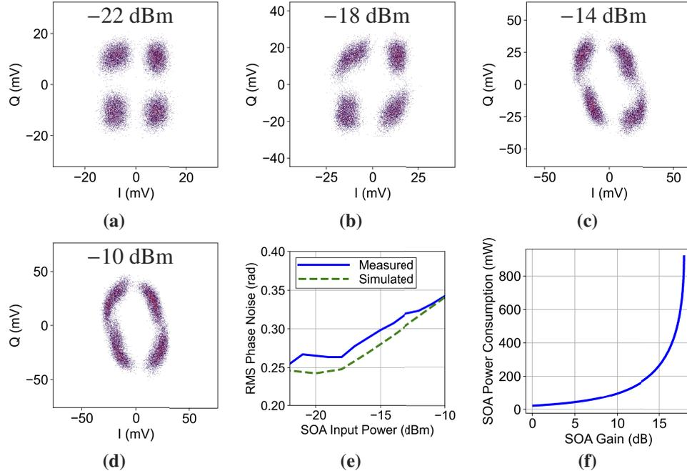
**Fig. 2.** Measured sampled QPSK constellations depicting the SOA pattern effect and NLPN for SOA input power levels of  $-22$  dBm (a),  $-18$  dBm (b),  $-14$  dBm (c), and  $-10$  dBm (d). (e) Measured vs modeled RMS phase error for various SOA input power levels. (f) Simulated SOA power consumption  $P_{soa}$  vs saturated gain  $G$ .
