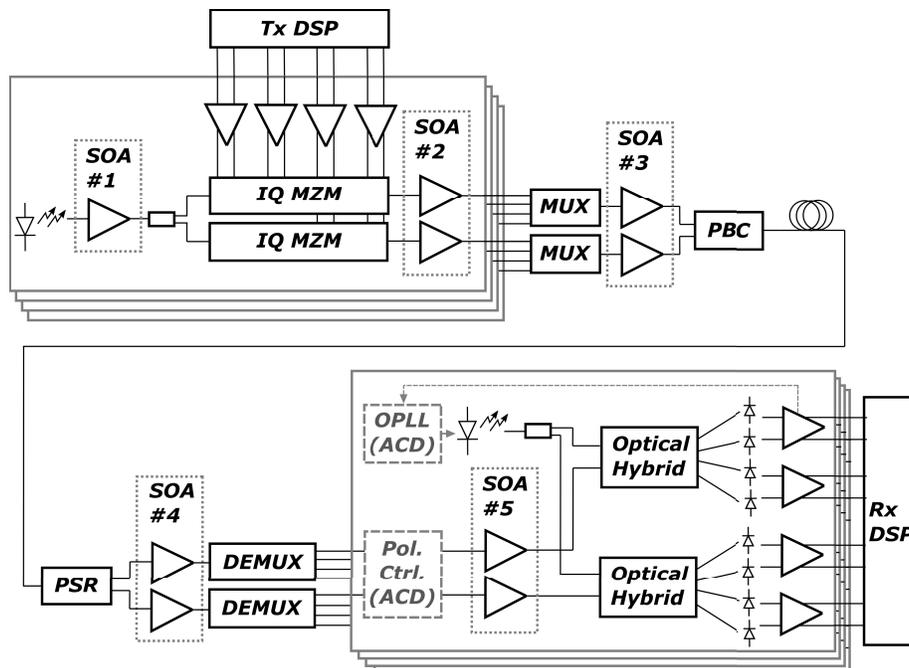
**Fig. 1.** General coherent link architecture. Boxes labeled SOA #1-5 indicate potential SOA insertion points throughout the link. The optical phased locked loop (OPLL) and polarization controller (Pol. Ctrl.) are used in ACD-based links, but omitted for conventional DSP-based ones.
