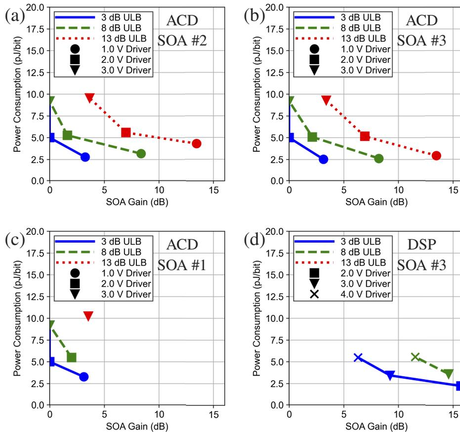
**Fig. 3.** Driver and SOA Power consumption vs. SOA gain for an ACD-based link with SOA in position #2 (a), #3 (b), and #1 (c), and for a DSP-based link with SOA in position #3 (d), where each curve corresponds to a particular supported ULB, and the differential peak-to-peak driver output voltages are marked.
