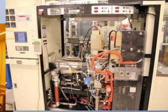
Panasonic ICP Etcher/Asher Dielectrics, Metals, Semiconductors Workhorse systems – often >18 Hrs/day nm-scale control - reproducible
