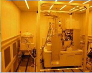
JEOL 6300 EBL Sub-10nm Patterning <5nm Stitching errors Full Wafers THz electronics Advanced Photonics
