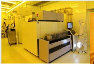
ASML-DUV-248nm Only 3 at Universities Sub-200nm Full Wafers Si-Photonics Quantum Computing
