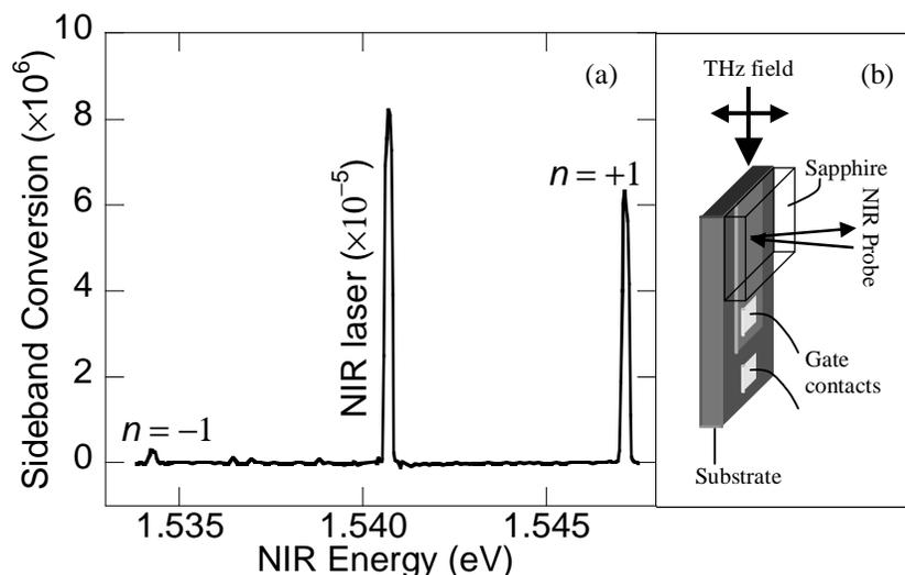
Fig. 1. (a) Sideband spectrum taken at 15 K with an FEL frequency of 1.5 THz (6.4 meV). The reflected beam at  $\omega_{\text{NIR}}$  is multiplied by  $10^5$ . The THz power was approximately 500 W and the NIR power was 0.67 mW. (b) The experimental geometry.
