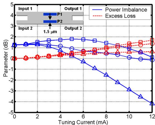
(c) Design 3. The tuning pads are each  $100\ \mu\text{m}$  long,  $1.5\ \mu\text{m}$  wide, and are placed in the center of the MMI region along the length and  $1\ \mu\text{m}$  from the edges along the width.
