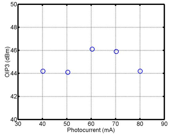
Fig. 5. Two-tone OIP3 as a function of photocurrent level.
