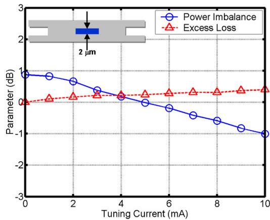
(b) Design 2. The tuning pad is  $100\ \mu\text{m}$  long,  $2\ \mu\text{m}$  wide, and is placed in the center of the MMI region.
