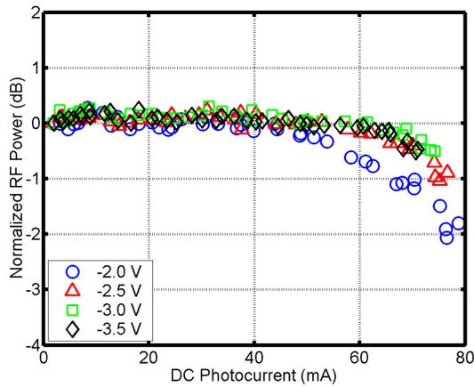
Fig. 3. Normalized RF power as a function of DC photocurrent at 1 GHz for varying bias voltages. The data is normalized to an ideal line with a slope of 20 dB/decade.
