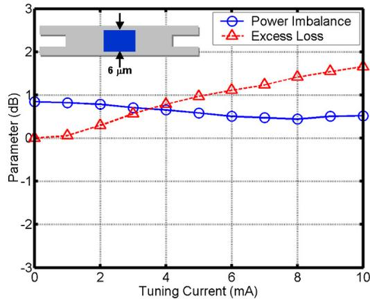
(a) Design 1. The tuning pad is  $100\ \mu\text{m}$  long,  $6\ \mu\text{m}$  wide, and is placed in the center of the MMI region.
