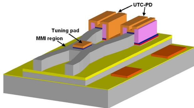
Fig. 1. Plan view schematic of UTC-BPD.
