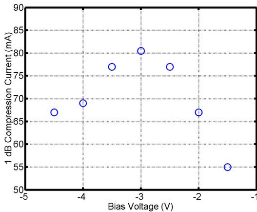
Fig. 4. 1 dB compression current as a function of bias voltage at 1 GHz.
