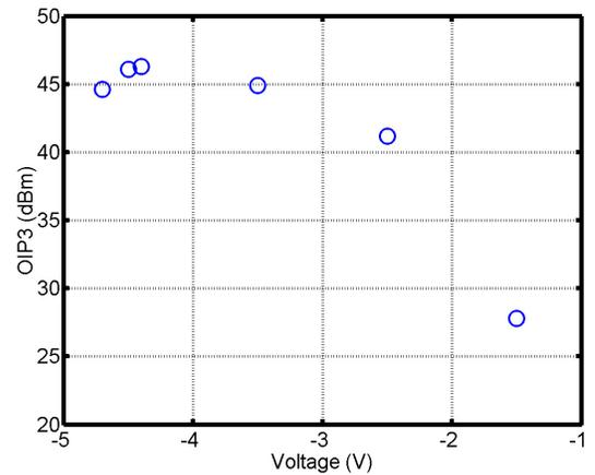
Fig. 6. Two-tone OIP3 as a function of bias voltage for a photocurrent level of 60 mA.
