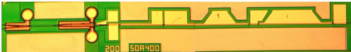
Integrated SGDBR-PD/SOA/MZI with data and data out 2000-2004
