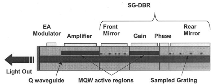
Fig. 1. SGDBR-SOA-EAM device schematic.
