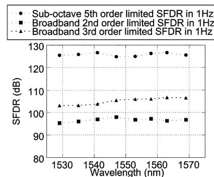
Fig. 5. Measured suboctave and broad-band spurious-free dynamic range, left scale, normalized to 1-Hz bandwidth for different wavelengths. Suboctave SFDR is measured at the third-order inflection point and limited by fifth-order intermodulation products. Broad-band SFDR is measured at the second-order inflection point and is limited by second- and third-order intermodulation products.
