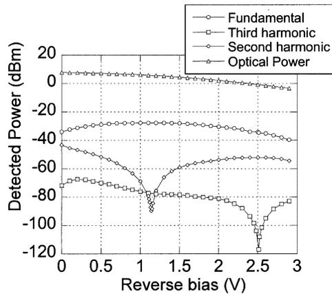
Fig. 3. Measured power of fundamental, second-, and third-order intermodulation products together with optical output power for 0-dBm modulation and 1545 nm.
