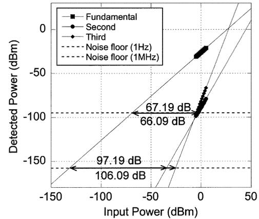
Fig. 4. Measured power of noise floor, fundamental, second-, and third-order intermodulation products at 1552 nm, for  $-5$ - to  $5$ -dBm input RF power, 6.3-mW optical power, and  $-1.1$ -V EAM bias. Broad-band SFDR is also shown in 1-Hz and 1-MHz bandwidth.
