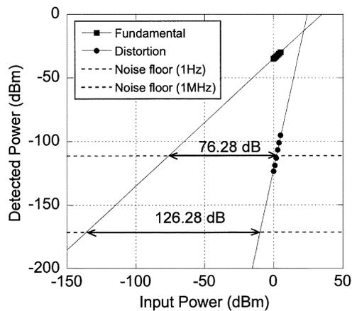
Fig. 6. Measured power of noise floor, fundamental, and third-order intermodulation products at 1552 nm, for 0- to 5-dBm input RF power, 0.96-mW optical power and  $-2.5$ -V EAM bias. Suboctave SFDR is also shown in 1-Hz and 1-MHz bandwidth.
