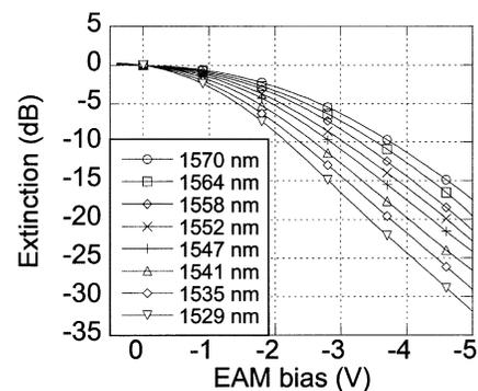
Fig. 2. EAM extinction over the tuning range of 1522–1573 nm.
