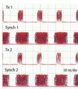
Fig. 7. Screenshots of transmitted and synchronized packets.
