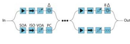
Fig. 4. Feed forward 4-stage optical packet synchronizer.
