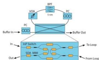
Fig. 5. Re-circulating optical packet buffer with inset of 2x2 InP switch.
