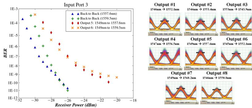
Figure 4. 40 Gbps BER measurements and eye diagrams for input port #3 and various output ports.
