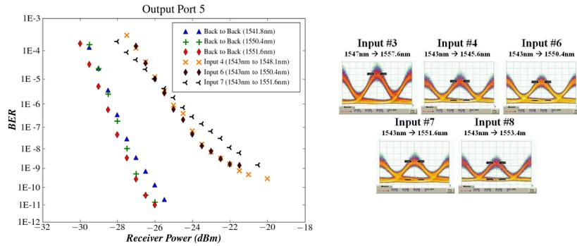
Figure 3. 40 Gbps BER measurements and eye diagrams for various input ports monitored at output port #5.
