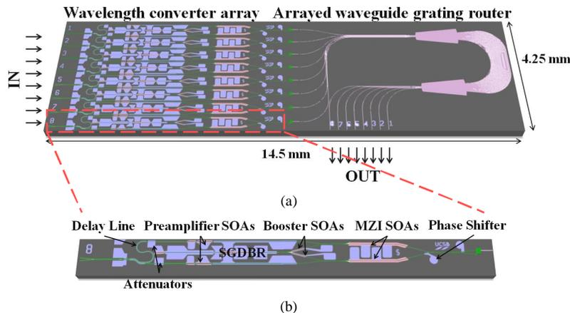
Figure 1. Schematic of the MOTOR chip: (a) overall device; (b) close-up of the wavelength converter design.
