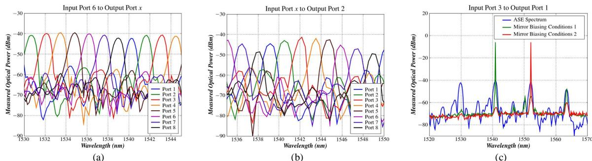
Figure 2: Output response of the integrated AWGR: (a) measured optical output from all output ports using input WC port #3; (b) measured optical output from output port #2 using each input WC port; and (c) lasing spectra for different biasing conditions using the SG-DBR of input WC port #3 superimposed on the ASE spectrum for that channel, all measured from output port #1.
