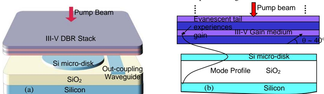
Fig. 1. (a) Schematic of a Si micro-disk coupled to III-V gain medium. The pump beam ( $\sim 1.31 \mu\text{m}$  in our experiments) enters from the top of the stack. The laser light is out-coupled through the waveguide, which is also used for Q measurements. (b) Cross-sectional schematic of the device.  $\theta$  represents the angle at which the evanescent light enters the III-V. The separation between the Si and the III-V stack is of the order of a few 100 nm.
