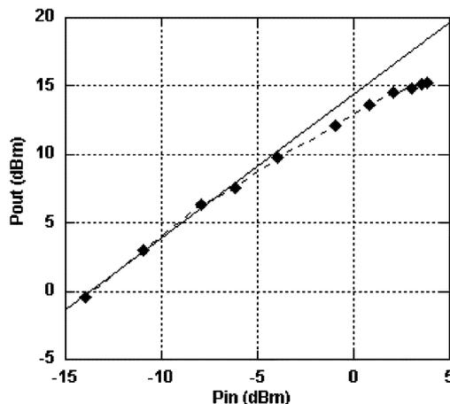
Fig. 5. Optical  $P_{\text{in}}$  versus optical  $P_{\text{out}} \propto I_{\text{photocurrent}}$  at 10 Gb/s. ( $I_{\text{SOA}} = 250$  mA ( $8.33$  kA/cm<sup>2</sup>) and  $V_{\text{detector}} = -4$  V).
