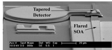
Fig. 1. Scanning electron microscope (SEM) of integrated photoreceiver.
