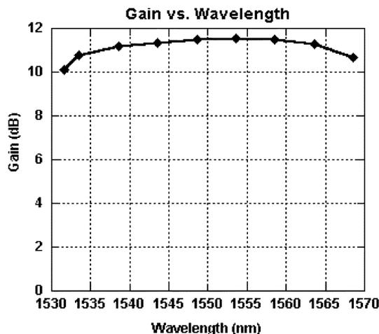
Fig. 2. Gain versus wavelength plot for receiver. ( $I_{\text{SOA}} = 250$  mA ( $8.33$  kA/cm<sup>2</sup>),  $V_{\text{detector}} = -4$  V, and  $P_{\text{in}} = 0.8$  mW).
