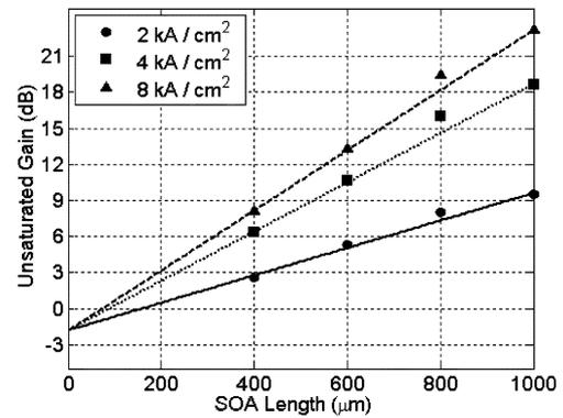
Fig. 8. Unsaturated gain versus length for three different current densities.
