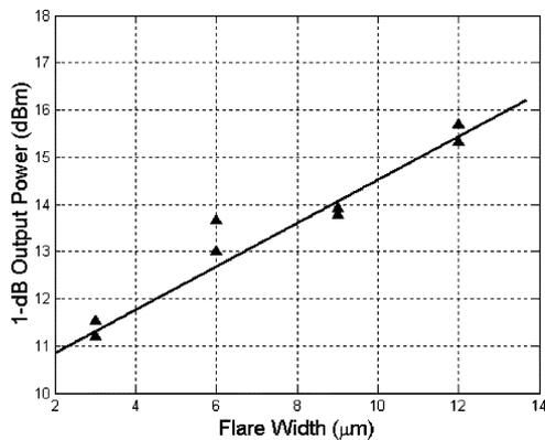
Fig. 7. Output power for 1-dB gain compression point versus the final flare width. ( $J_{\text{SOA}} = 8.33$  kA/cm<sup>2</sup>).
