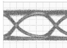
Fig. 4. 20-Gb/s eye for  $2^{31}$ -1 pseudorandom binary sequence (PRBS). ( $I_{\text{SOA}} = 250$  mA,  $V_{\text{detector}} = -5$  V, and  $P_{\text{in}} = 0.8$  mW).
