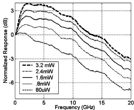
Fig. 3. Input power dependence of the frequency response of the receiver. ( $I_{\text{SOA}} = 250$  mA ( $8.33$  kA/cm<sup>2</sup>) and  $V_{\text{detector}} = -4$  V).
