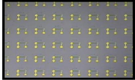
Monolithic MEMS-based tuning Single cavity VCSEL-based laser VCSELs tested at a wafer levels before substantial cost and time expended to determine wafer yield
