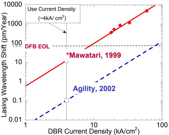
\*Mawatari et al, "Lasing Wavelength Changes Due to Degradation in Buried Heterostructure DBR Laser", Journal of Lightwave Technology, v.17, no.5 1999
