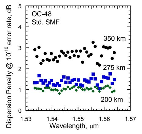
Dispersion penalty at 10<sup>-10</sup> errors/s error rate for 200, 275, and 350 km of standard SMF for 38 ITU channels sampled across C-band.
