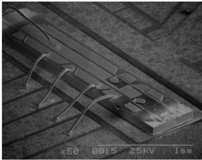
Fig. 2. Electron micrograph of transmitter device.
