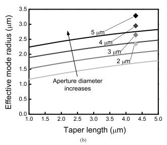
Fig. 7. (a) Round-trip optical scattering loss and (b) effective mode radius versus taper length for different device sizes, ranging from 2 to 5  $\mu$ m in diameter. These curves were calculated assuming the effective indices in the unoxidized and fully oxidized sections are 3.254 and 3.113, respectively. Superimposed are the simulated results for the original taper aperture, plotted as circles (scattering loss) in (a) and diamonds (effective mode radius) in (b).
