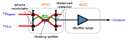
Figure 2. 'All-optical' coherent receiver for phase modulated signals. (No EIC in feedback path)
