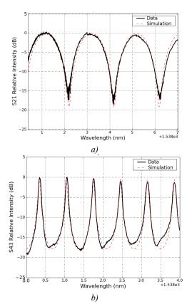
Fig. 4 Measured Single Unit Cell responses with superimposed  $S_{21}$  simulations using (1). a) MZI zero response; b) Resonator pole response.
