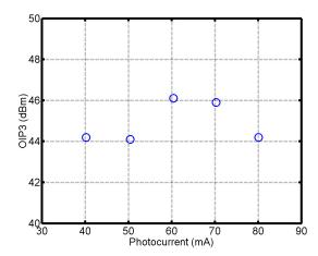
Fig. 5. Two-tone OIP3 as a function of photocurrent level.
