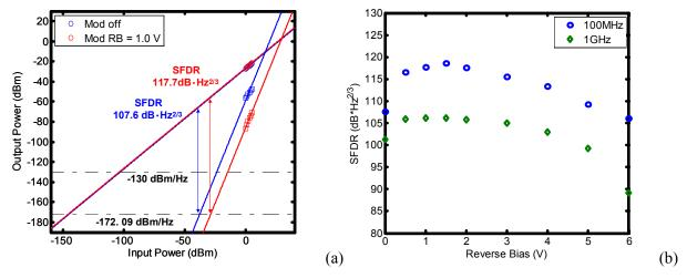
Fig. 3 (a) The two-tone measurement at 100 MHz with modulator off and reverse bias at 1 V. (b) Shot noise limited SFDR results versus different modulator reverse biases at 100 MHz and 1 GHz.
