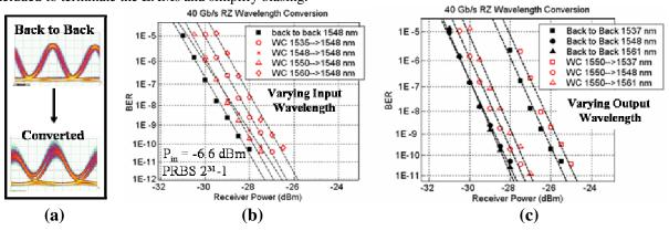
Fig 2. (a) 40 Gb/s back-to-back (1550 nm) and wavelength converted eye diagrams (1550  $\rightarrow$  1548 nm) (b) Wavelength converted BER measurements for varying input wavelength and (c) varying output wavelength compared with back-to-back transmission.
