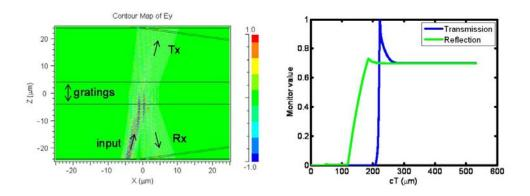
Fig. 4. FDTD simulation of the Bragg grating splitter with one input at equal splitting condition. (a) FDTD color-coded contour plot of the optical field. (b) Time monitor outputs at transmission and reflection versus time in units of cT ( $\mu$ m) where c is the speed of light in vacuum.
