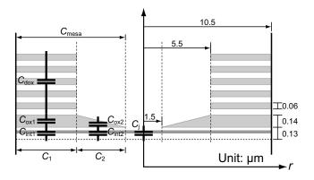
Fig. 17. Various components for  $C_{\rm mesa}$  in our devices. The lengths are labeled for 3  $\mu m$  diameter devices.
