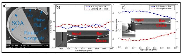
Fig. 1a. SEM of fabricated SRL with MMI coupler, 1b/c. MMI/zero-gap coupler splitting ratio vs. wavelength
