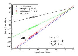
Figure 5. Calculated IMD3 and IMD2 ( $P_{dc}$ = 40mW)
