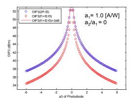
Figure 9. OIP3 dependence on  $a_3$  of photodiode with  $a_2/a_1 = 0$  but not a perfectly linear optical source  $(c_2/c_1 = -0.01 \text{ and } c_3/c_1 = -0.001)$
