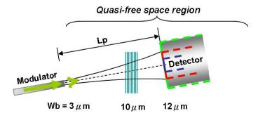
Fig. 8. Beam divergence in the quasi free space region. The beam waist is 3 \_m at the input from modulator, 10 \_m at the grating region, and 12 \_m at the detector front end. Di\_erent detector widths are also illustrated in blue (S), red (M), and green (L).
