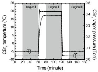
Fig. 2: The CBr<sub>4</sub> temperature and vapor pressure with the temperature setpoint changed between -5°C and 20°C
