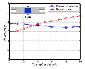
(a) Design 1. The tuning pad is 100  $\mu$ m long, 6  $\mu$ m wide, and is placed in the center of the MMI region.
