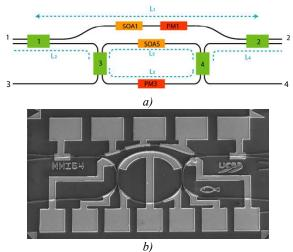
Fig. 2 a) Schematic and b) SEM picture of the Single Ring Unit
