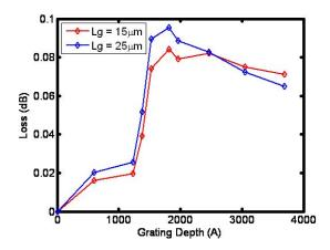
Fig. 7. The FDTD simulated loss versus grating etch depth in the vertical model. Total slab waveguide thickness is 3695 \_A.
