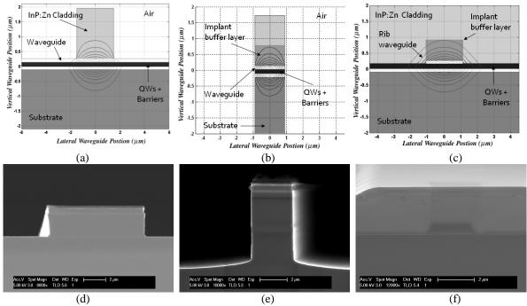
Fig 3. Ridge architectures used in MOTOR: (a), (b), (c) show schematic cross-sections of epitaxial layers with the optical mode profile superimposed for surface ridge, deep ridge, and buried rib, respectively. (d), (e), (f) show corresponding SEM cross sections for surface ridge, deep ridge, and buried rib, respectively
