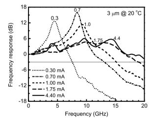
Fig. 3 Frequency responses for 3  $\mu m$  device at 20°C under different bias currents
