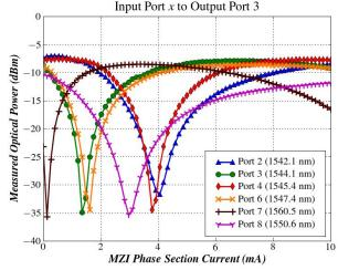
Fig. 6. MZI transfer functions for six of the eight input wavelength converters measured from output port #3
