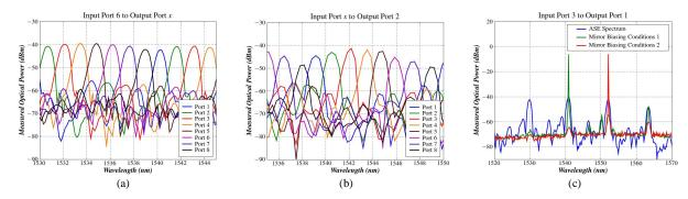
Figure 2: Output response of the integrated AWGR: (a) measured optical output from all output ports using input WC port #3; (b) measured optical output from output port #2 using each input WC port; and (c) lasing spectra for different biasing conditions using the SG-DBR of input WC port #3 superimposed on the ASE spectrum for that channel, all measured from output port #1.
