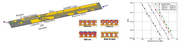
Fig. 3. All-photonic widely-tunable wavelength converter that integrates an SGDBR-SOA-TW/MZM transmitter with a two-stage SOA-PD receiver. NRZ-Eye diagrams and bit-error-rate @ 40Gb/s illustrated for 1550 nm input data across 32 nm. Power penalties similar for different input wavelengths. Equivalent circuit is similar to Fig. 2 (a) except MZM diodes connected in series push/pull across PD [10].
