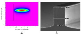
Fig.1 a) Simulated mode profile for deep etched ridge. b) SEM image of deep etched ridge waveguide.
