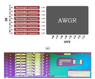
Fig. 1. a) Schematic overview of MOTOR architecture; (b) Photograph of fabricated device
