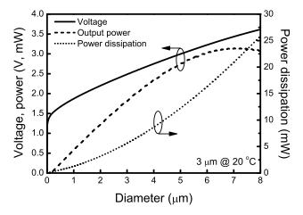
Fig. 13. L-I-V-P curves for 3 μm devices at 20°C.
