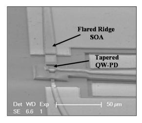
Fig. 11. SEM of the receiver depicting the flared ridge SOA followed by the high-power QW PD.
