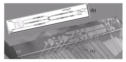
Figure 1 - 40 Gbps packet forwarding chip (a) Schematic representation of nonlinear SOA-based CAM device; (b) Optical micrograph of a fabricated CAM device.
