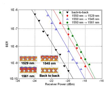
Figure 4 - Bit error rate measurements for 40 Gbps RZ input data for the Mach-Zehnder SAM wavelength converter
