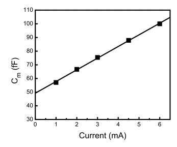
Fig. 18. Extracted  $C_{\rm m}$  versus the bias current for 3  $\mu m$  device.
