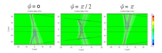
Fig. 5. FDTD simulation of the grating splitter with two inputs in different phase relations.
