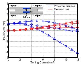
(c) Design 3. The tuning pads are each 100  $\mu m$  long, 1.5  $\mu m$  wide, and are placed in the center of the MMI region along the length and 1  $\mu m$  from the edges along the width.
