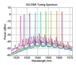
Fig. 8. Overlaid output spectra of nine supermodes from the SG-DBR laser.
