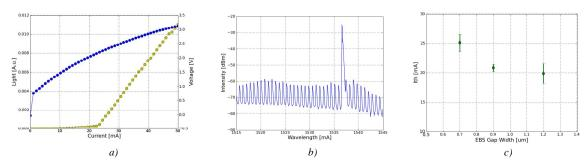
Fig.4 a) LIV characteristic for an EBS ring resonator. b) Lasing spectra for same device at 65mA. c) Threshold currents as a function of EBS gap width, mean values and standard deviations indicated.
