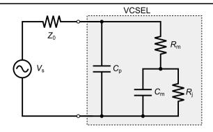
**Fig. 6** Small-signal equivalent circuit model for the device. The device is represented by  $C_{\rm p}$ ,  $R_{\rm m}$ ,  $C_{\rm m}$ , and  $R_{\rm j}$ .  $V_{\rm s}$  is the RF voltage source and  $Z_0=50~\Omega$  is the characteristic impedance of the instruments
