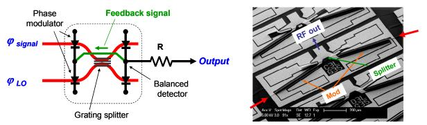
Fig. 1 Schematic and SEM of the integrated all-photonic receiver.
