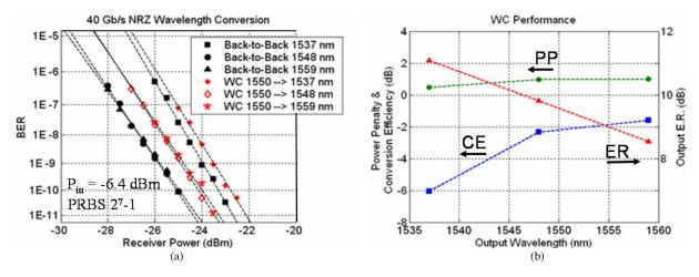
Fig. 18. (a) 40 Gb/s BER measurements for fixed input wavelength and varying output wavelength for input power of -6.4 dBm. (b) Measured power penalty (PP), output extinction ratio (ER), and conversion efficiency (CE) versus output wavelength.
