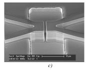
Fig 2. a) RIE-lag limits the EBS gap depth. b) Multiple-thickness SiO<sub>2</sub> mask effectively delays the waveguide deep etch. c) RIE-lag is reduced yielding higher aspect ratio EBS gaps
