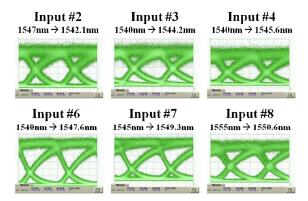
Figure 2: 10 Gbps eyes for the six working input channels measured out of output port #3.
