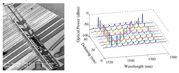
Fig.2. Left) SEM of Integrated OPLL PIC. Right) Output spectra from heterodyne optical source.
