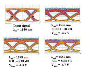
Fig. 19. 40 Gb/s NRZ input and wavelength-converted eye diagrams corresponding to the BER measurements in Fig. 18. Gate bias and output extinction are listed.
