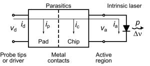
Fig. 1. Cascaded two-port model of diode laser.
