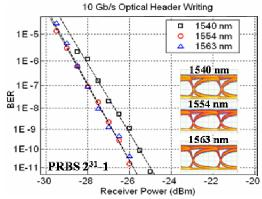
Fig 3. BER measurements for 10 Gb/s NRZ optical label writing for varying SG-DBR wavelengths. Insets show corresponding eye diagrams with 2.0 V peak-to-peak drive.
