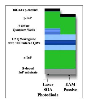
Fig. 4. DQW integration platform. The layer structure chosen for each region of the chip is denoted.
