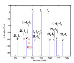
Figure 2. Ilustration of IMD3 components in a three-tone experiment
