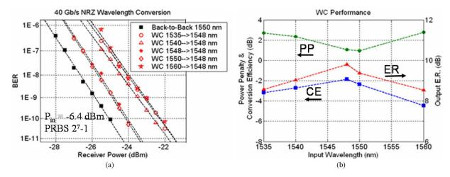
Fig. 17. (a) 40 Gb/s BER measurements for varying input wavelength and constant output wavelength for input power of -6.4 dBm. (b) Measured power penalty (PP), output extinction ratio (ER), and conversion efficiency (CE) versus input wavelength.
