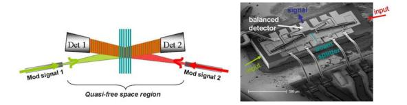
Fig. 1. (a) Schematic top view of 2x2 grating-based beam splitter which is integrated with two modulators and two photodetectors. Waveguide boundary (not shown) is far away from the diverged beams in the quasi free space region.
