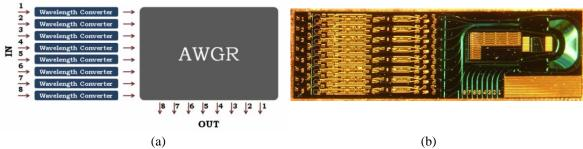
Figure 1. (a) Schematic overview of MOTOR architecture; (b) Photograph of fabricated device.
