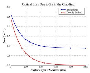
Fig. 4. Effect of the implant buffer layer thickness on the scattering loss due to Zn doping in a buried rib and deeply etched waveguide (model assumes no Zn diffusion)
