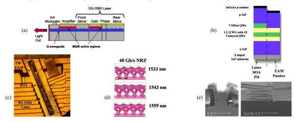
Fig. 1. (a) Vintage SGDBR-SOA-EAM using off-set QW platform [6]; (b) dual-QW layer structure; (c) mounted SGDBR-SOA-TW/EAM; (d) digital eyes across at several wavelengths; (e) TW/EAM waveguide cross section and top-view perspective [7].
