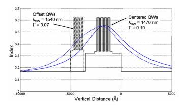
Fig. 5. Index and optical mode profile for the "active" (dotted) and "passive" (solid) regions of the device.
