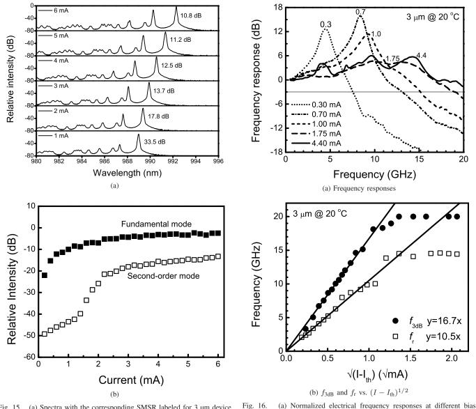
Fig. 15. (a) Spectra with the corresponding SMSR labeled for 3 µm device at different bias currents. (b) The intensities for the fundamental and second-order modes versus bias current.
