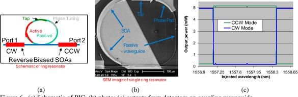
Figure 6. (a) Schematic of PIC; (b) photo; (c) outputs from detectors on coupling waveguide.
