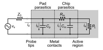
Fig. 3. Small-signal model with the driving source. The VCSEL is grayed.
