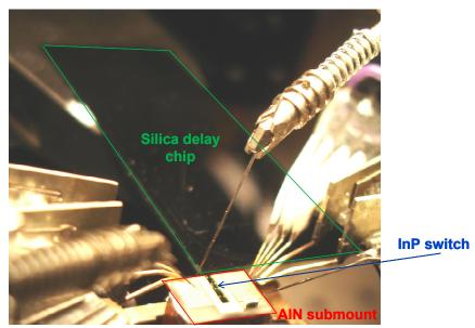
Figure 11 – Photograph of the optical buffer used in LASOR architecture – InP switch and the silica delay line chip
