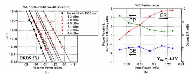
Fig. 16. (a) 40 Gb/s BER measurements for wavelength conversion from 1550 to 1548 nm for varying optical input power compared with back-to-back transmission. (b) Measured power penalty (PP) at BER of  $10^{-9}$ , output extinction ratio (ER), and facet-to-facet conversion efficiency (CE) at each input power.
