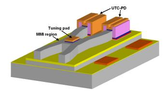
Fig. 1. Plan view schematic of UTC-BPD.
