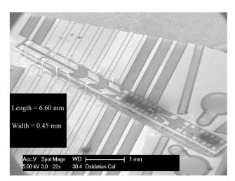
Figure 2. An SEM image of a fully fabricated OPLL-PIC after mounting on a test-carrier and wire-bonding.
