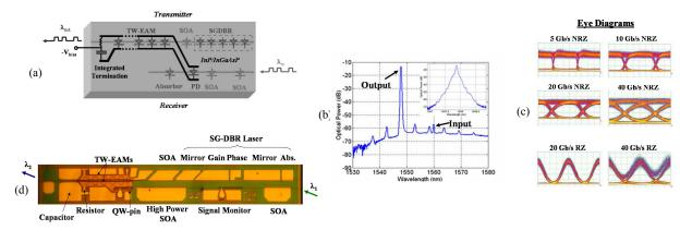
Fig. 2. (a) Functional schematic of all-photonic transceiver; (b) unfiltered unmodulated (and inset modulated @ 40Gb/s - expanded across 1.7 nm) output spectrum; (c) digital eyes for RZ and NRZ modulation from 5-40 Gb/s; (d) photo of transceiver with SGDBR-SOA-TW/EAM transmitter and two-stage SOA—PD receiver[9].
