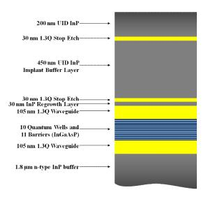
Fig. 2. Epitaxial base structure for quantum well intermixing
