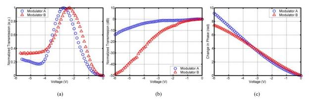
Figure. 4. (a) Normalized MZM transmission, (b) normalized EAM transmission, and (c) phase change as a function of bias voltage.
