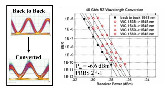
Figure 8 - Bit error rate measurement results for 40 Gbps RZ input data for the traveling wave EAM SAM wavelength converter
