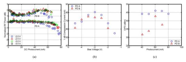
Figure. 2. (a) Normalized RF power as a function of DC photocurrent at 1 GHz. The data for PD A is normalized to 0 dB and that for PD B to 2 dB. (b) 1-dB compression current as a function of bias voltage. (c) Two-tone OIP3 as a function of photocurrent.
