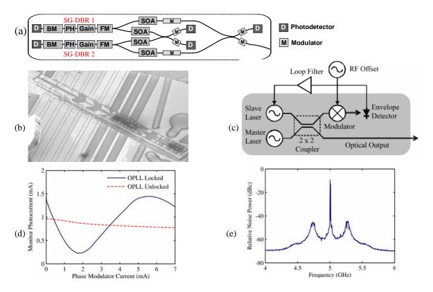
Figure 7. (a) Chip schematic); (b) chip SEM; (c) Circuit showing chip, feedback and offset modulation elements; (d) non-offset comparison of monitor current [detector on far right] as phase of reference laser is tuned [via the lowest central modulator]; (e) output spectrum for a 5GHz rf offset signal applied.
