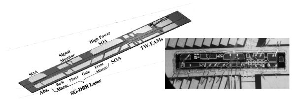
Figure 5 - 40 Gbps packet forwarding chip – Schematic representation of the traveling wave EAM field-modulated SAM device and an optical micrograph of a chip on carrier.
