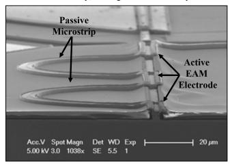
Figure 7 - Periodically loaded microstrip lines, designed to provide better matching in group velocities between the optical and electrical signals
