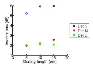
Fig. 11. Measured insertion loss data versus grating lengths.
