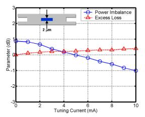
(b) Design 2. The tuning pad is 100  $\mu$ m long, 2  $\mu$ m wide, and is placed in the center of the MMI region.
