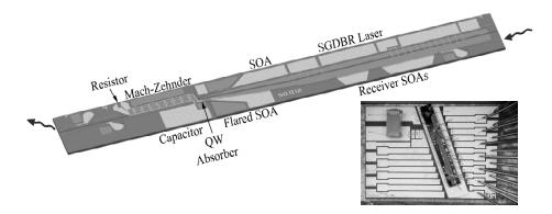
Figure 2 - 40 Gbps packet forwarding chip – Schematic representation of the Mach-Zehnder modulator field-modulated SAM device and an optical micrograph of a chip on carrier.
