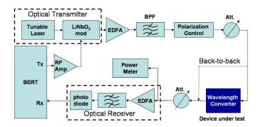
Fig. 15. Measurement setup for characterization of the wavelength conversion performance. BER of converted signal is compared to back-to-back transmission for varying power into the optical receiver.
