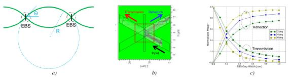
Fig 1. a) Schematic illustration of flattened ring resonator design. b) EBS design and 2D-FDTD simulation. c) Simulated power splitting as a function of incident angle and gap width.
