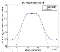
Fig.5 Measured and simulated throughput from 2-coupledring bandpass filter tuned to  $\sim 0.1$  dB ripple with a 0.302 nm (37.7 GHz) FWHM.
