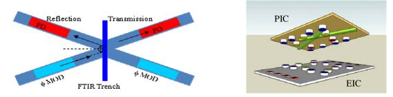
Figure 3. FTIR Trench coupler PIC configuration and flip-chipping concept.
