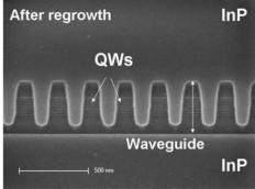
Fig. 3. (a) Schematic side view of the grating region. The beam is only confined in vertical direction. (b) Regrown gratings cross-section. The slab waveguide layer which contains multiple centered quantum wells can be clearly seen. No obvious air void is observed at the regrowth interface.
