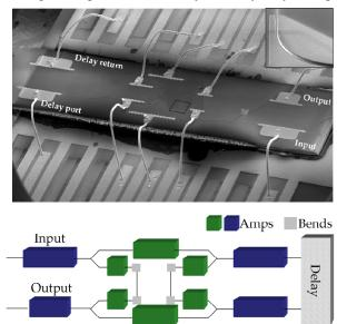
Figure 9 - Schematic of 2x2 switch with amplifiers (bottom) SEM image of the switch affixed and wire-bonded to a submount (top)
