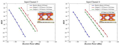
Figure 4: BER measurements for input channels 3 and 4. BERs are measured from two different output ports for each input port. Power penalties at a BER of 10<sup>-9</sup> range from 3.2 to 4.4 dB.
