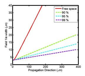
Fig. 2. Comparison of field 1/e width of quasi free space expansion and linear flaring along propagation direction. Different mode expansion speeds in linear flaring give different power transfer percentages (e.g. 90 %, 95 % and 99 %).
