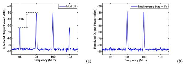
Fig. 2 Receiver output power spectra at 100 MHz, 10 mA photocurrent. (a) Modulator turned-off. (b) Modulator reverse-bias at 1 V.
