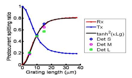
Fig. 10. Photocurrent splitting ratio versus grating length. Lines are from modeling and circles are the measured data.
