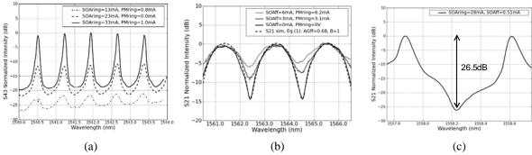
Figure 5. (a),(b) Isolated pole and zero responses tuned in amplitude by varying bias on feed-forward SOA and ring SOA respectively, the ring phase modulator is used to fix the filter in frequency. (c) Zero and pole are utilized simultaneously to enhance extinction ratio.
