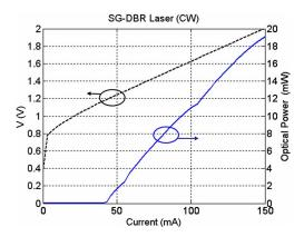
Fig. 7. SG-DBR laser LIV characteristic.
