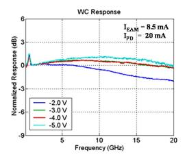
Fig. 14. Small-signal optical-to-optical response of the wavelength converter.
