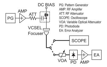
Fig. 19. Experiment setup for bit error rate and eye diagram.
