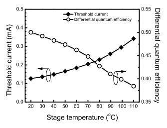
Fig. 14. Threshold current and differential quantum efficiency versus stage temperature for 3  $\mu$ m diameter devices.
