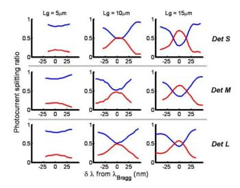
Fig. 9. Measured splitting spectra of nine di\_erent combinations with di\_erent detector widths and di\_erent grating lengths. Red (lower) lines represent the reection and blue (upper) lines represent the transmission.
