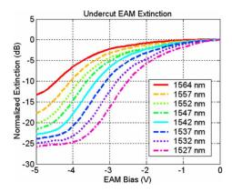
Fig. 10. DC extinction characteristic for the 250- $\mu$ m TW-EAM over the tuning range of the SG-DBR.
