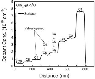
Fig. 3: Doping profile measured by SIMS with eight different valve combinations
