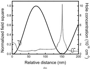
Fig. 6. (a) Grading and doping and (b) normalized electric field square and simulated hole concentration in one DBR period.
