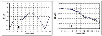
Fig. 2a: Return loss S11 of chip-on-carrier with a  $750\mu m$  long modulator. Fig. 2b: Electro-optical response of chip-on-carrier with a  $750\mu m$  long modulator.
