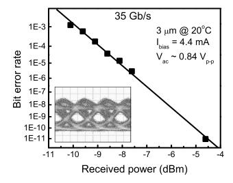
Fig. 20. Bit error curve at 35 Gb/s for 3  $\mu m$  diameter device. The device was biased at 4.4 mA and a RF voltage swing of 0.84  $V_{p-p}$  was used. The inset shows the corresponding optical eye diagram with an extinction ratio of 5.4 dB.
