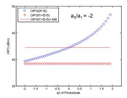
Figure 6. OIP3 dependence on  $a_2$  of photodiode
