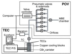
Fig. 1: Schematics of the CBr<sub>4</sub> doping system
