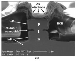
Fig. 9. SEMs of a high-impedance TW-EAM structure. (a) Periodic microstrip electrode design. The modulator has been cleaved halfway along the length. (b) Cross section of the ridge waveguide with selectively undercut intrinsic region for low capacitance.
