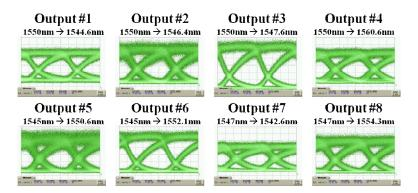
Figure 3: 10 Gbps eyes using input channel #6 measured out of every output port.
