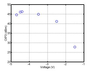
Fig. 6. Two-tone OIP3 as a function of bias voltage for a photocurrent level of 60 mA.
