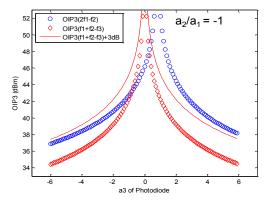
Figure 7. OIP3 dependence on  $a_3$  of photodiode
