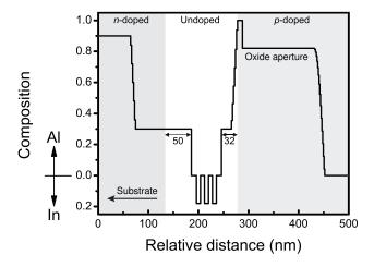
Fig. 10. Cavity structure of our devices.
