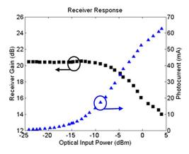
Fig. 12. Measured receiver gain and generated photocurrent as a function of input power.
