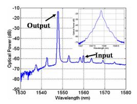
Fig. 20. Output optical spectrum from the wavelength converter demonstrating 45 dB input suppression. Inset shows higher resolution plot of the output signal with 40 Gb/s modulated data spectrum.
