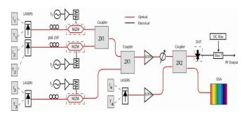
Figure 1. Experimental setup: three-tone measurement
