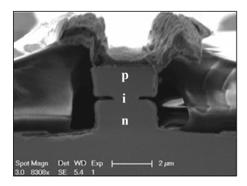
Figure 6 – Travelling wave modulator cross section, showing the undercut waveguide design
