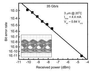
**Fig. 5** Bit error rate curve at 35 Gb/s for 3  $\mu$ m diameter device. This device was biased at 4.4 mA and a RF voltage swing of 0.84  $V_{p^-p}$  was used. The inset shows the corresponding optical eye diagram with an extinction ratio of 5.4 dB
