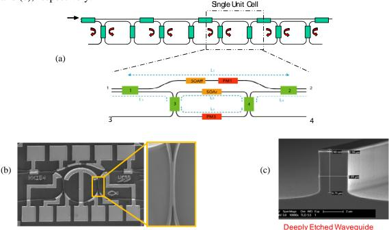
Figure 4. (a) Ring-resonator-based lattice filter and unit cell; (b) topview of fabricated filter unit cell together with blow-up of directional coupler; (c) deeply-etched waveguide crossection.
