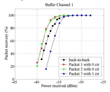
Figure 10 – Packet recovery rate as function of received power for buffer tested at 40 Gbps RZ
