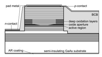
Fig. 4. schematic cross-section of our devices.
