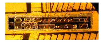
Fig. 13. Photograph of DUT mounted and wirebonded to an AlN carrier.
