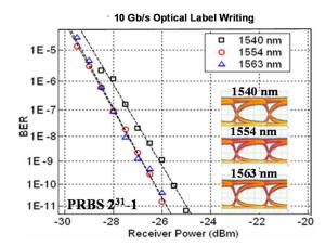
Fig. 21. BER measurements for external modulation of label-writing EAM at 10 Gb/s. Eye diagrams at each wavelength are shown.
