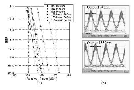
Figure 3 – CAM PFC: (a) Bit error rate results for 40 Gbps RZ wavelength conversion; (b) Eye diagram for an output wavelength of 1550 nm.
