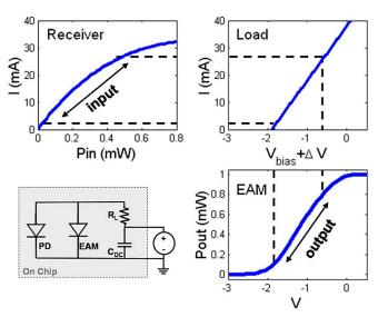
Fig. 3. Example of the three-part transfer function for the field-modulated optical gate. Circuit diagram is shown in the lower left.
