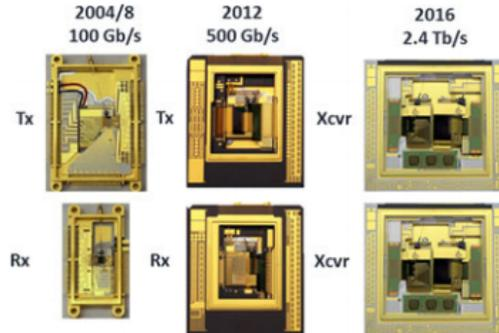
Fig. 21. Scaling of four generations of multi-channel DWDM SOC photonic IC modules. From their first commercial deployment in 2004 to 2016 (12 years), the data capacity of these modules has scaled 24x in roughly the same footprint (images shown to scale).
