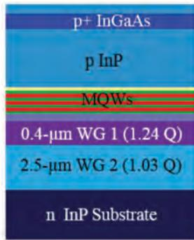
Fig. 2. Epitaxial structure of the InP-based transmitter with a low-index dilute waveguide ( $1.03 \text{ Q}$ ).
