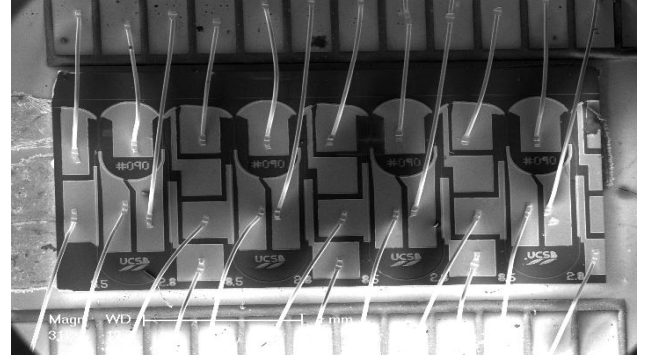
Figure 2. Scanning electron microscope image of a fabricated device containing four unit cells; device has been wirebonded to a carrier.
